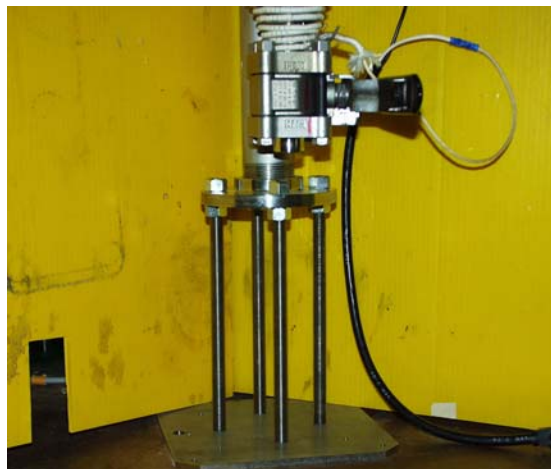
Fig II. The Bottom Valve of the ANL-Designed LEU-Foil Digester
