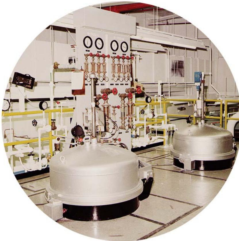
**Figure I. Induction Furnace**
