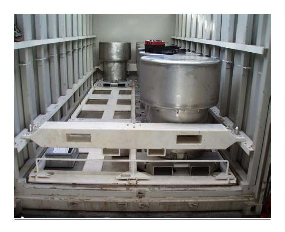
The **TN-CIEL** is an innovative concept of mobile tank vehicle type IP2, intended for road transportation of waste radioactive and potentially corrosive liquids:
