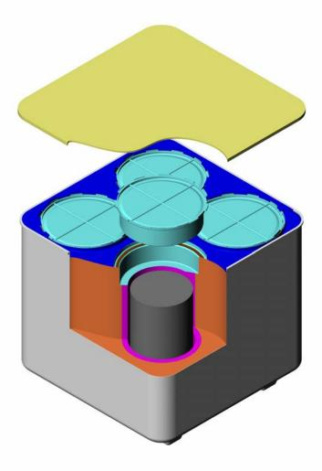
The TN-MTR presents a cylindrical cavity, in which today 7 different kinds of baskets are available to comply with the characteristics of the spent fuel to be shipped.
