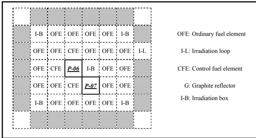
Figure 1: Core Configuration
