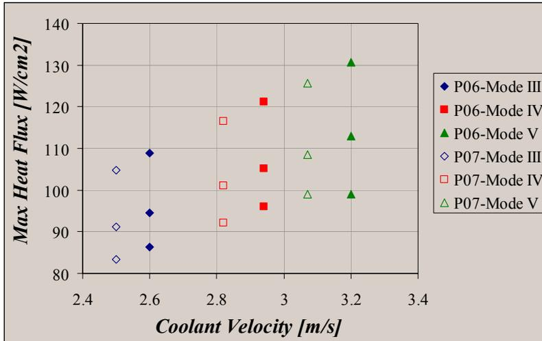
Figure 3: Max. heat fluxes for each prototype and operating mode
