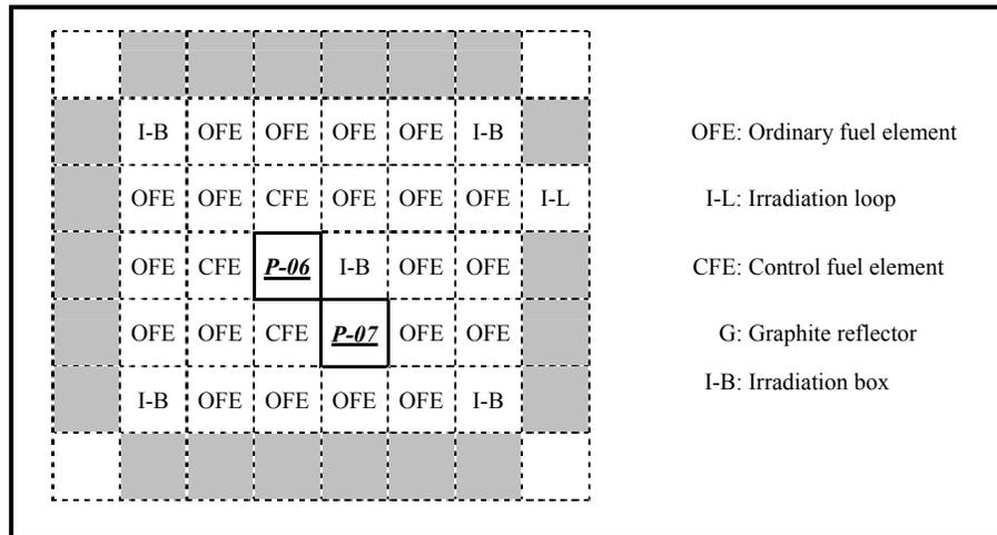
Figure 1: Core Configuration
