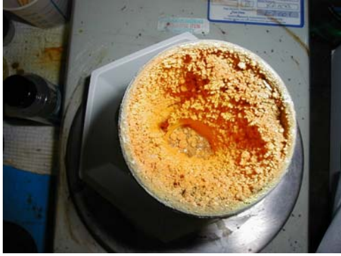
Figure III. Photograph of the calciner cup after feed of 675 g U (1420 g UNH) in 6.68 L of 1 M nitric acid solution was completed.
