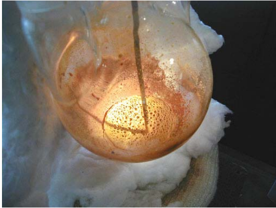
Figure V. Photograph of the reaction flask after feed was stopped and all of the liquid was boiled away. The lighting was arranged to highlight the porous, yellow solid in the bottom of the vessel.
