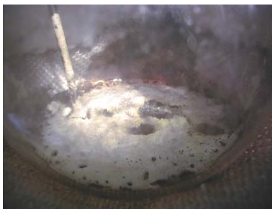
Figure VIII. Photograph of the reaction vessel some time after all of the liquid was evaporated. The temperature of the system was about 450°C.
