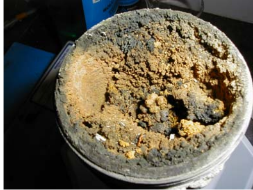
Figure IV. Photograph of the calciner cup calcination (600°C for 2 hours) of the material shown in Figure III.
