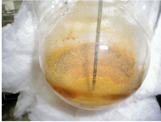
Figure VI. Photograph of the reaction flask after feed was stopped and all of the liquid was boiled away. The lighting was arranged to highlight the splatter on the side of the vessel.
