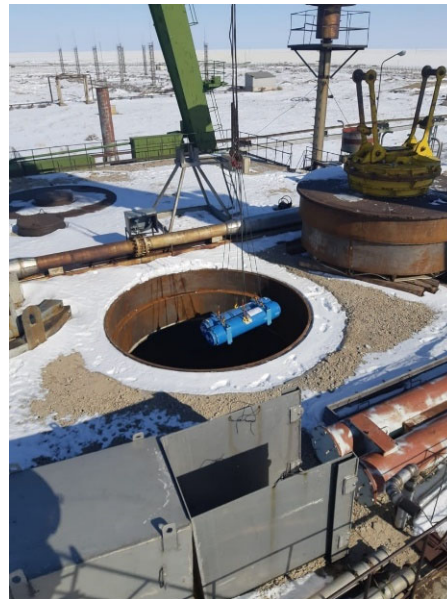
Loading of LEU fuel into IVG.IM storage
