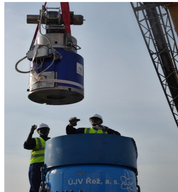
Transfer cask with HEU inside
