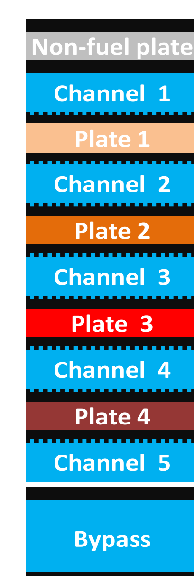
Schematics and Geometry of the Fuel Assembly (Total Input Power = 2 MW)
