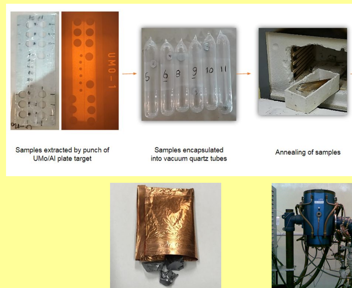
Figure 2. Phase transformation test: Thermal treatment of samples of UMo plate type target Below, vacuum thermal treatment of U-10 wt% Al alloy lumps, wrapped into copper envelope
