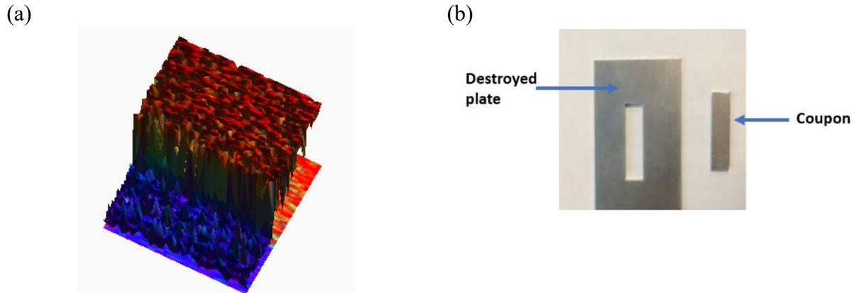
Fig.4 (a) 2D ultrasonic image of the interface; (b) Coupon extraction from the plate.
