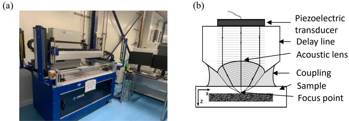
Fig.2 (a) OKOS acoustic microscope; (b) Functioning principle of a focused transducer.
