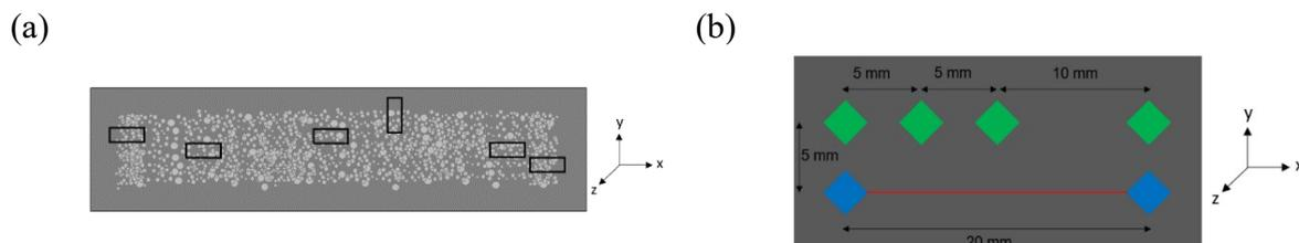
Fig.1 (a) Coupon to be analyzed in a plate; (b) Position of the indentations for each coupon.
