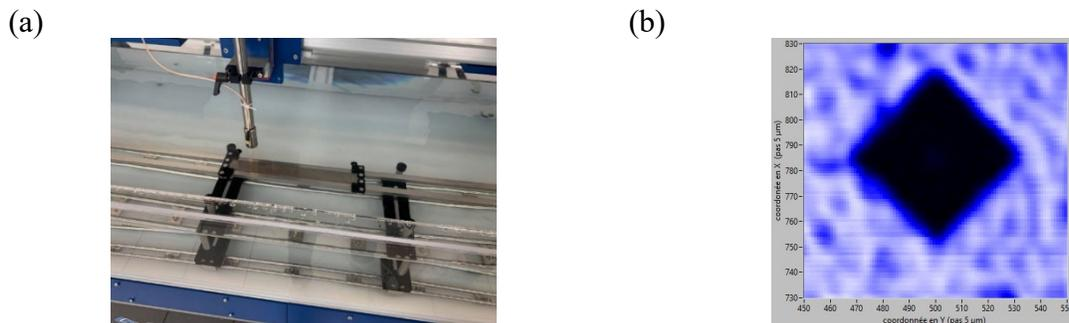
Fig.3 (a) Plates in the sample holder; (b) Ultrasonic image of one of the plate mark.
