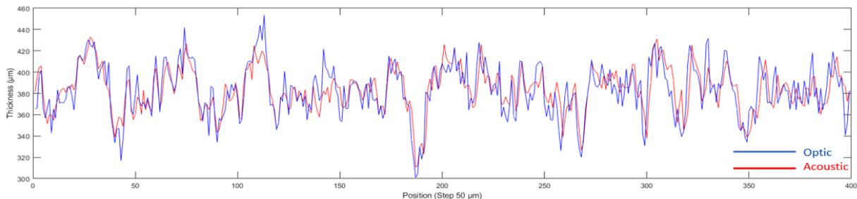
Fig.6 Optical and acoustic thickness measurement of the measuring line.
