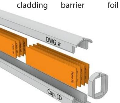
Capsules, each with 8 mini-plates, were irradiated in ATR in "B" positions and the South Flux Trap
