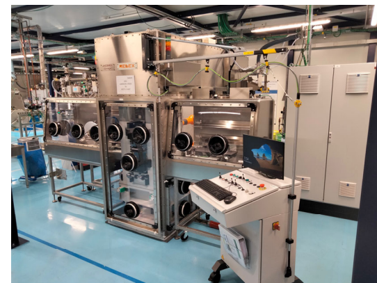
Figure 7: Cold rolling mill into glovebox
