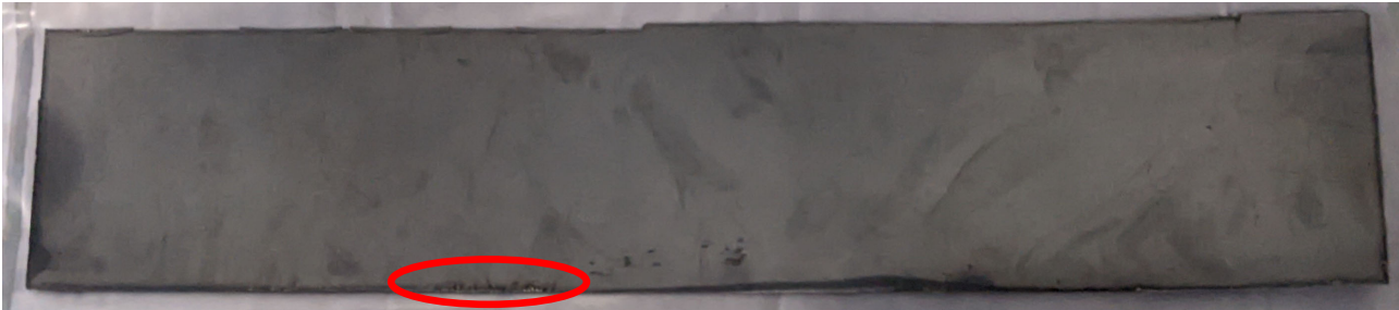
Figure 16: U-Mo bare foil defects after hot rolling process
