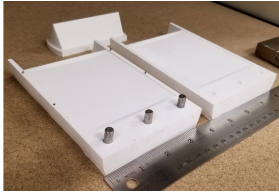
Figure 5. "clamshell" mold design example.
