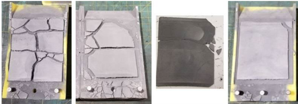
Figure 6. CIP fuel geometry parts which were cracked upon removal from CIP.
