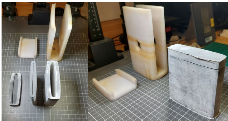
Figure 8. (Left) Full-size billet geometry mold with brace disassembled. (Right) Full fuel geometry mold assembled with brace disassembled.
