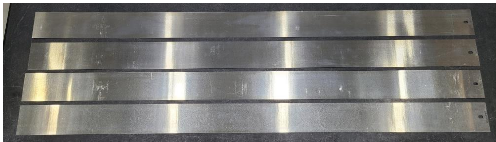
[Prototype of full-size 5.3 gU/cc U_3Si_2 flat fuel plate]
