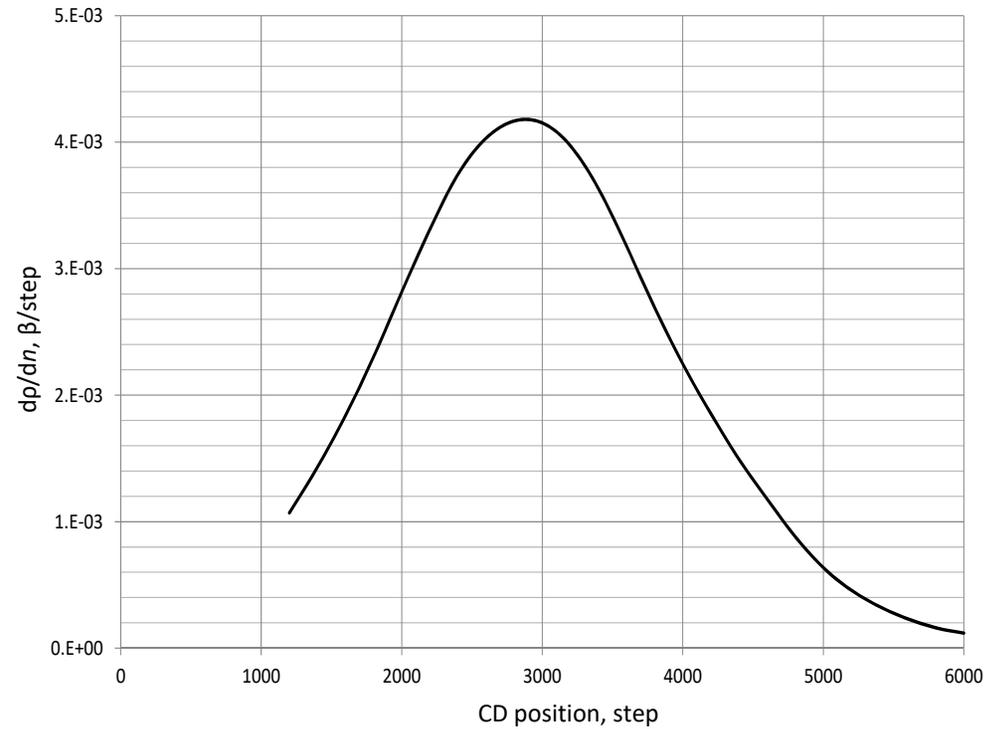
*Differential characteristic of Control Drums (CD) system*
