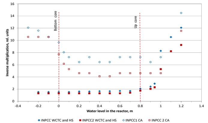
Countdown curves during filling with water of WCTC-LEU, thermal screens and the central assembly of the reactor
