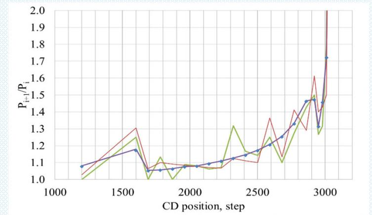
Comparison of the ratio of the impulse chambers readings between adjacent states and the ratio of the subcritical neutron multiplication factor (SMF)
