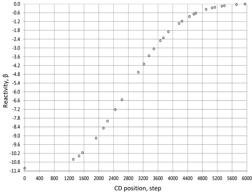
*Control characteristic of the Control Drums (CD) system*
