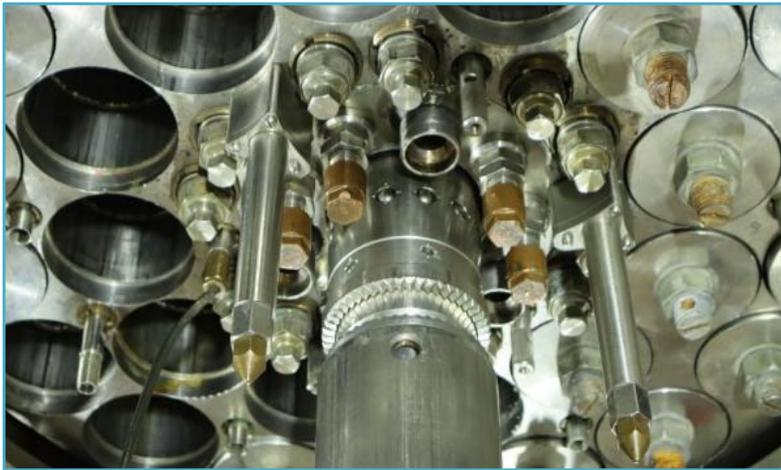
*Bottom view of the reactor. Loading of the physical experimental channel (PEC) in the central assembly 72.000*
