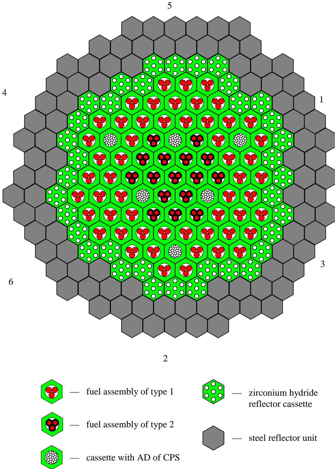
Figure 7. The loading configuration of the critical assembly 2
