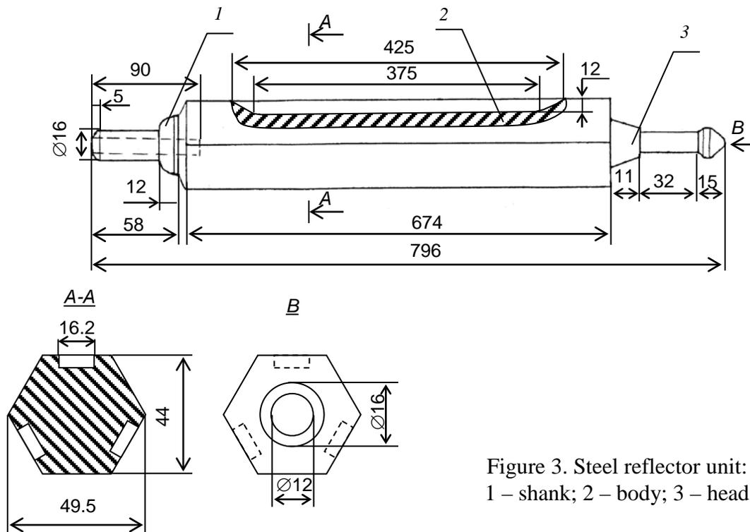
Figure 3. Steel reflector unit:
