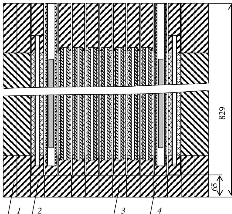
Figure 4. The analytical model of the critical assembly: 1 – analytical model steel reflector unit; 2 – analytical model zirconium hydride reflector cassette; 3 – analytical model of the fuel assembly; 4 – analytical model of the cassette with AD of CPS
