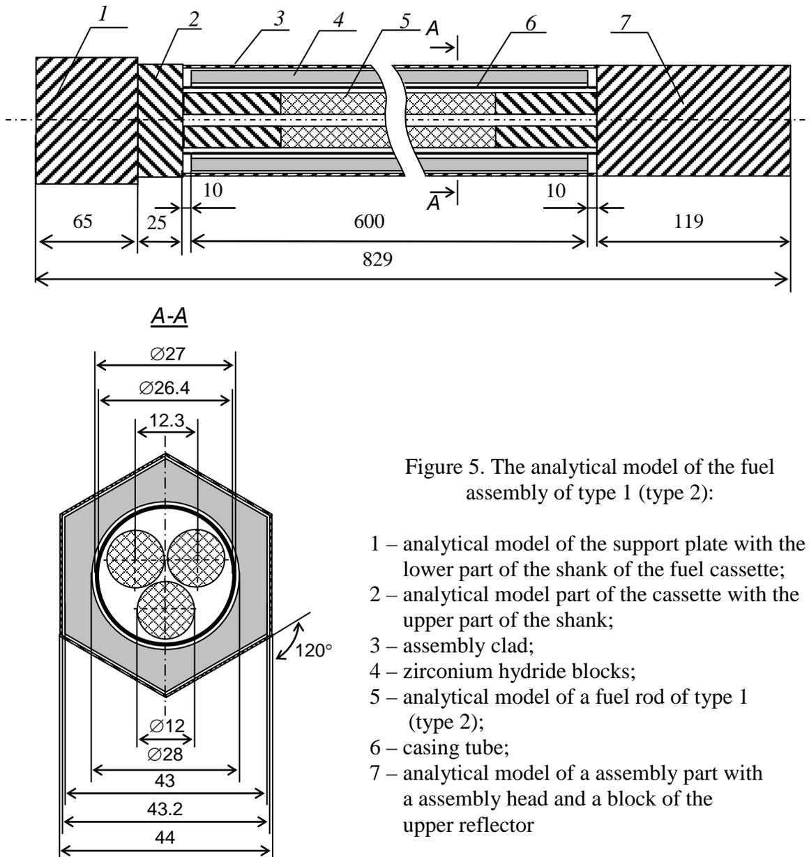
Figure 5. The analytical model of the fuel assembly of type 1 (type 2):
