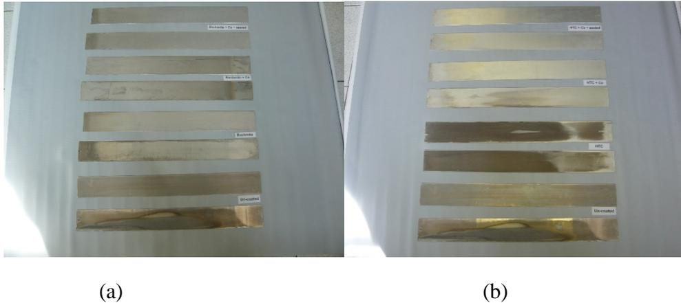
Figure 6. Photographs of full-size plate surfaces. (a) Boehmite coated and (b) HTC coated. The plates above the identification mark were exposed for 8 months and the plates below, for 14 months.
