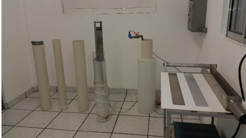
Figure 7. Setup to coat a dummy fuel element with HTC.
