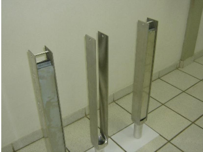
Figure 1: Photograph of plates assembled to form dummy fuel elements.
