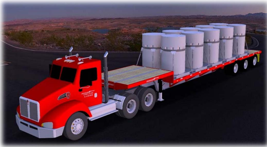
Fig. 3. Typical OPTIMUS™-L Package Transport Configuration
