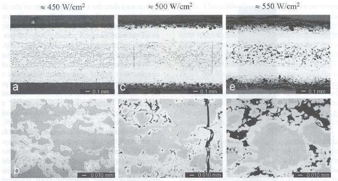
Figure 10: Images of the  $U_3Si_2$ -Al dispersion fuel showing the effect of fuel power (or temperature) [12].
