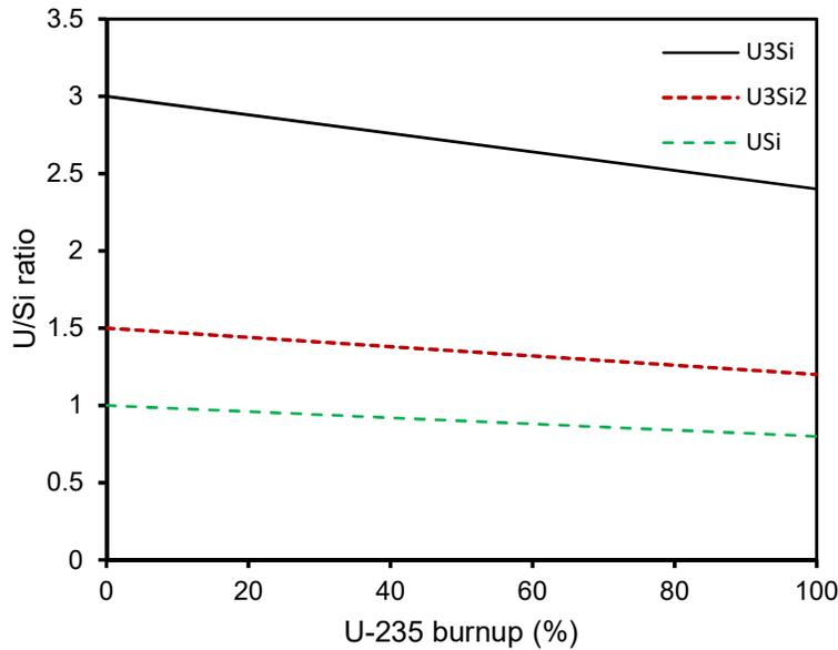
Figure 2: Change in U/Si ratio as uranium in 20% enriched uranium silicide is burned.
