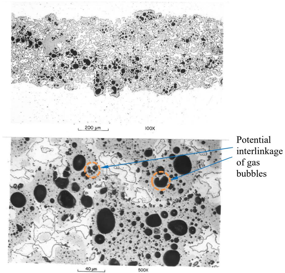
Figure 6: Microstructure of ORR Demonstration element CSI-202 at 97% burnup showing no fabrication porosity and early stage of linking of gas bubbles in some areas [1].
