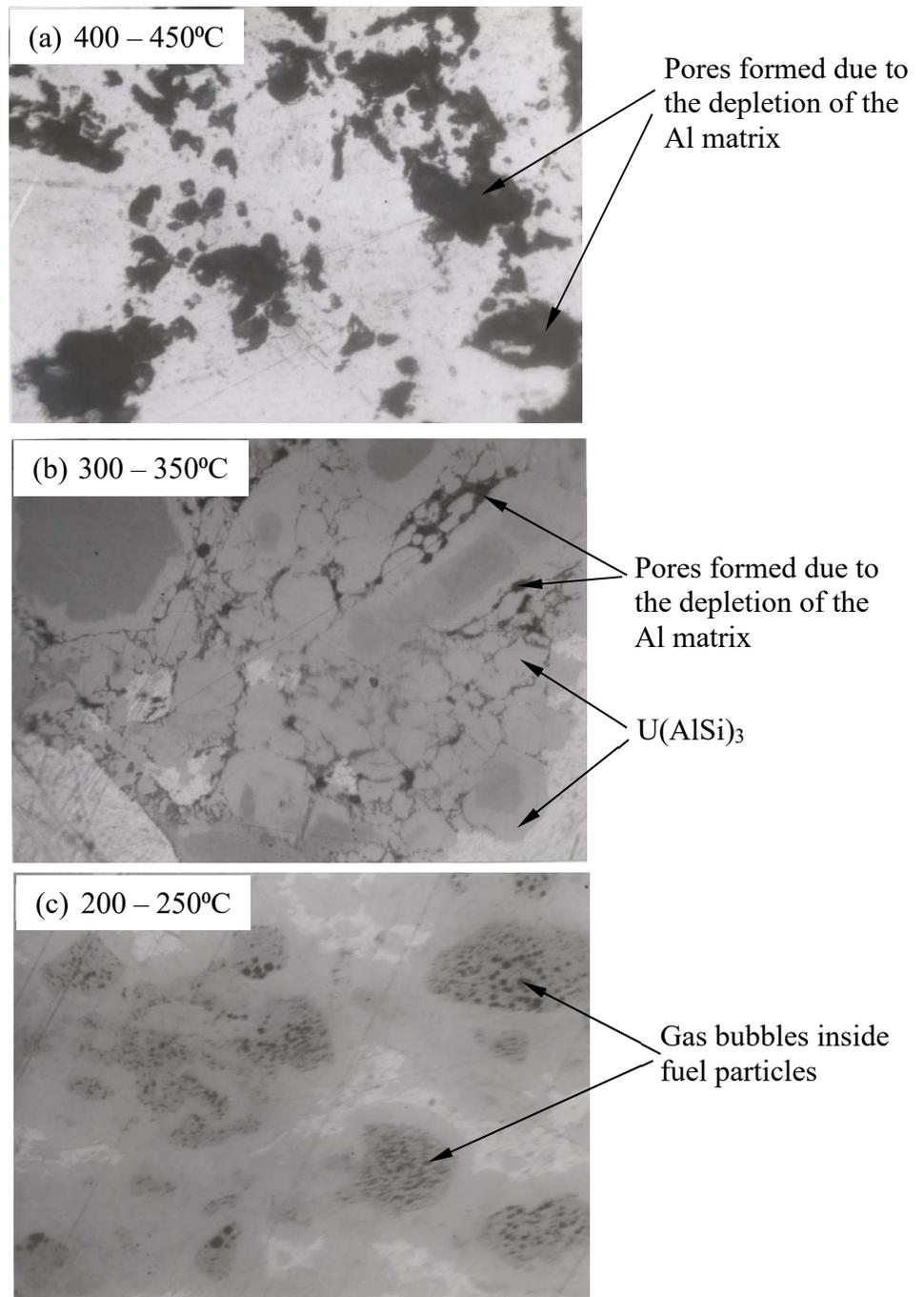
Figure 8: Low-enriched  $U_3Si_2$ ,  $4.8 \text{ g/cm}^3$  dispersion fuel samples irradiated in HFIR for one cycle of 22.9 EFPD to 74-91% U-235 depletion, at indicated fuel temperatures [8].
