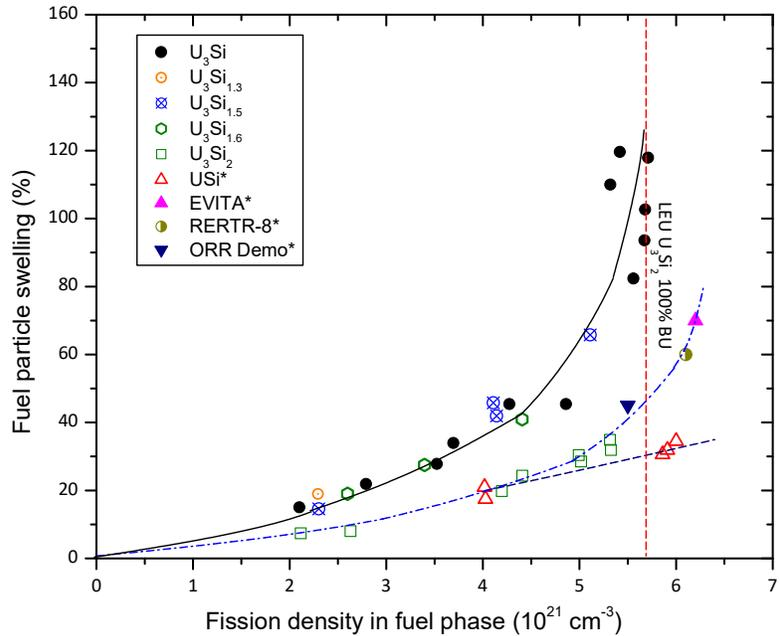
Figure 3: Fuel particle swelling in various U-Si/Al dispersion fuel plates (\* Enriched in U-235 higher than 20%). “EVITA” data is from Ref. [6], “RERTR-8” data is from Ref. [7], “ORR Demo” data is from Ref. [1], and other data sets are from Ref. [8].
