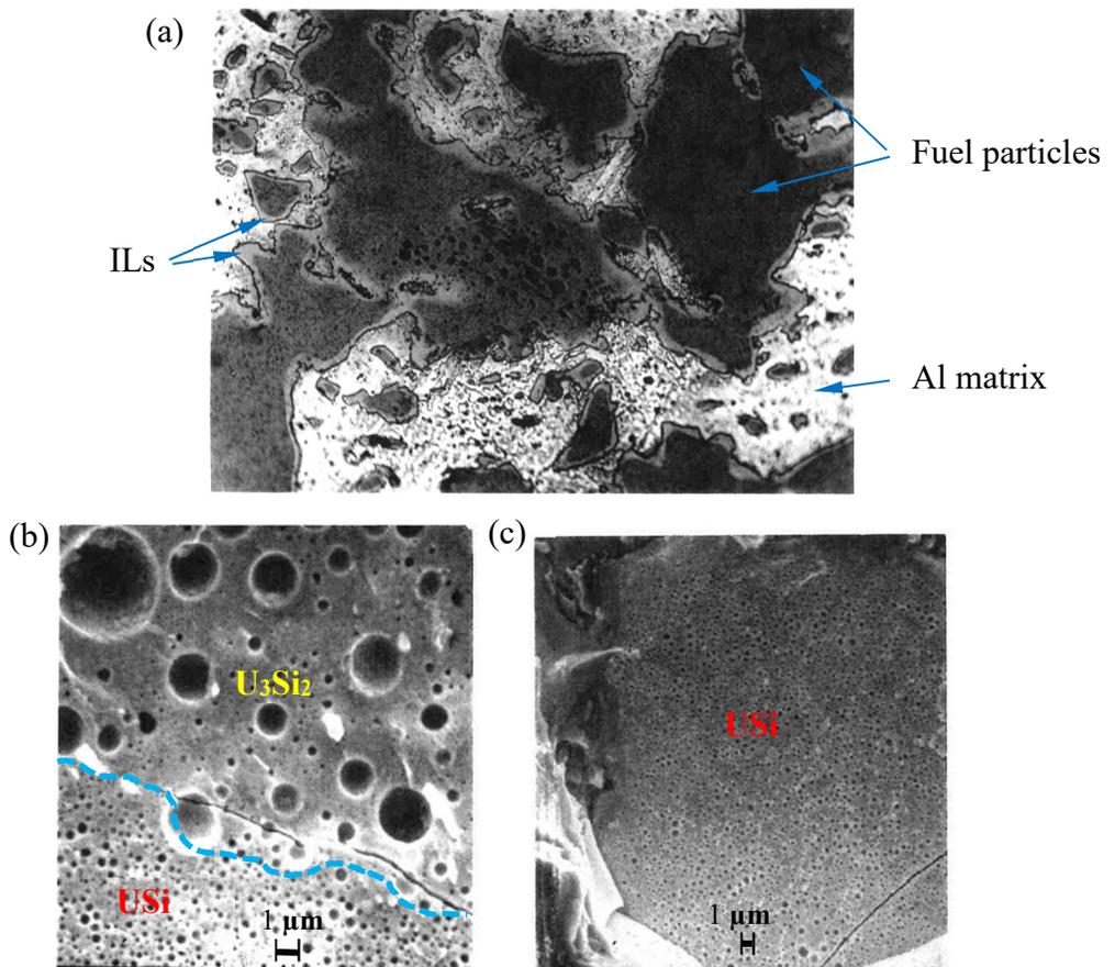
Figure 5: Micrographs of MEU  $USi$  irradiated to  $5.9 \times 10^{21}$  fission/cm<sup>3</sup> (65% LEU burnup): (a) overall microstructure, (b) microstructure of a region presumably composed of mixed  $U_3Si_2$  and  $USi$ , and (c) general fission gas bubble morphology of irradiated  $USi$ . Note that scale bars are different in (b) and (c).
