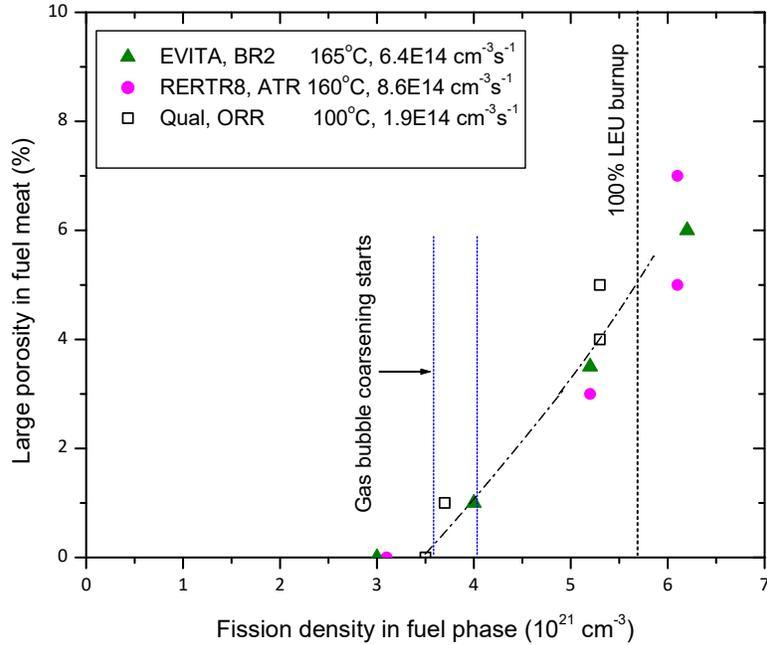
Figure 7: Coarsened fission gas bubble fraction in meat of various  $\text{U}_3\text{Si}_2$ -Al dispersion fuel plates. “EVITA” data is from Ref. [6], “RERTR8” data is from Ref. [10], and “Qual” data is from Ref. [1].
