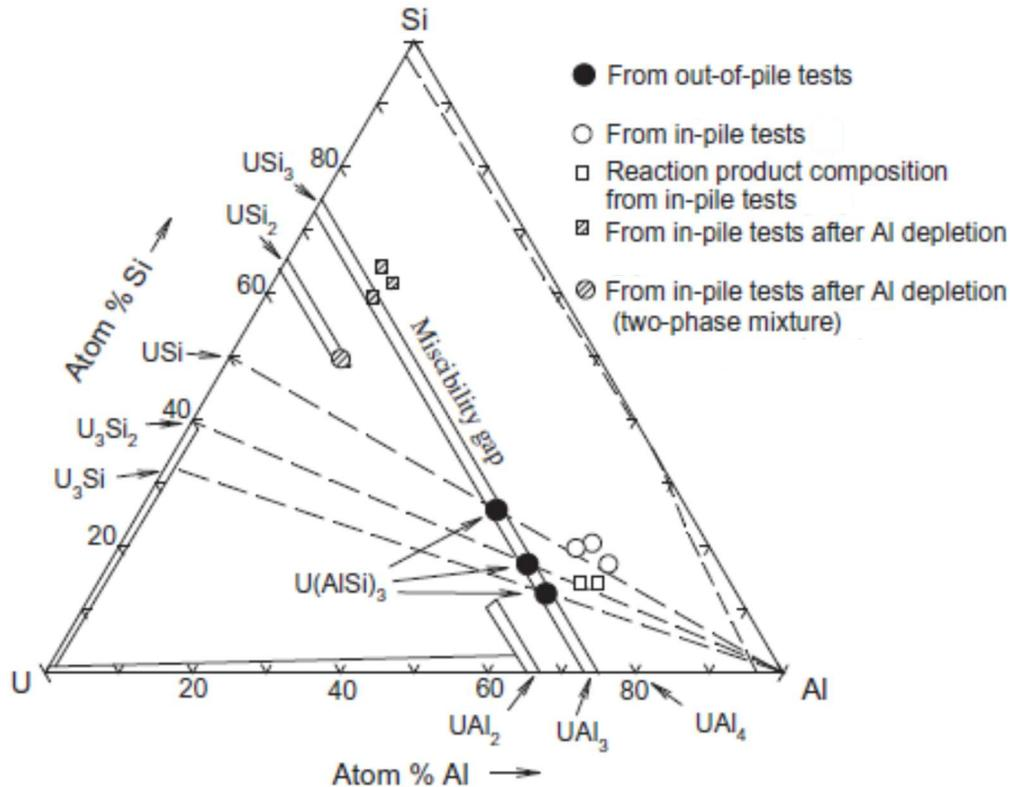
Figure 9: U-Si-Al ternary phase diagram showing compositions of reaction products between  $U_3Si_2$  and Al [11].
