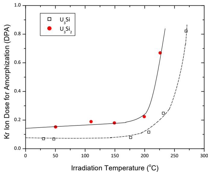
Figure 1: Temperature dependence of amorphization by ion irradiation of U-Si compounds. “U<sub>3</sub>Si” data is from Ref. [4] and “U<sub>3</sub>Si<sub>2</sub>” data is from Ref. [5].
