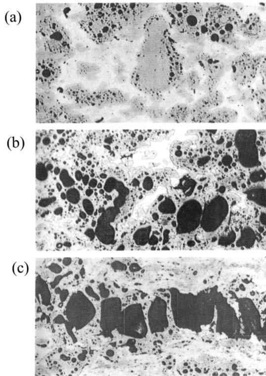
Figure 4: Fission gas bubble development in LEU  $U_3Si$  showing (a) initial swelling stage, (b) breakaway stage and (c) pillowing [9].
