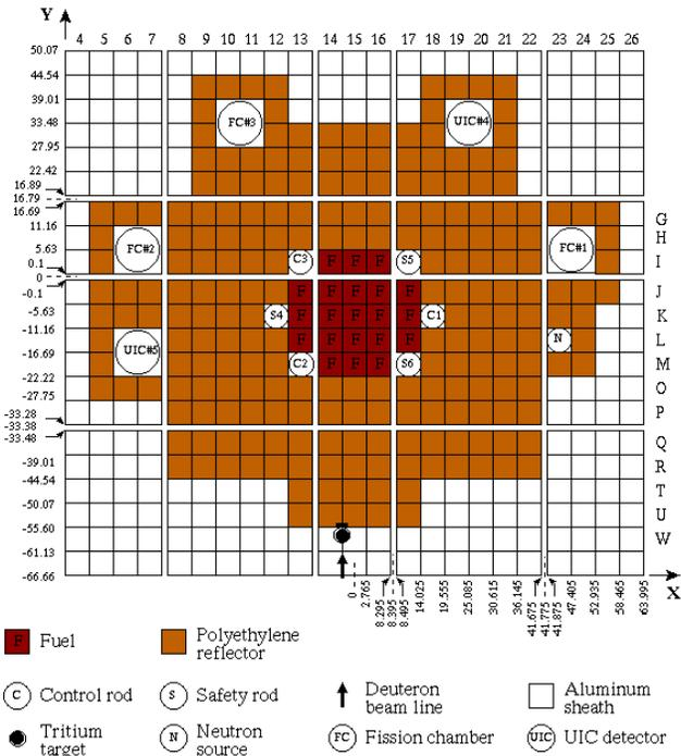
Figure 3. KUCA Dry Core Benchmark Assembly Configuration (A3/8"P36EU)
