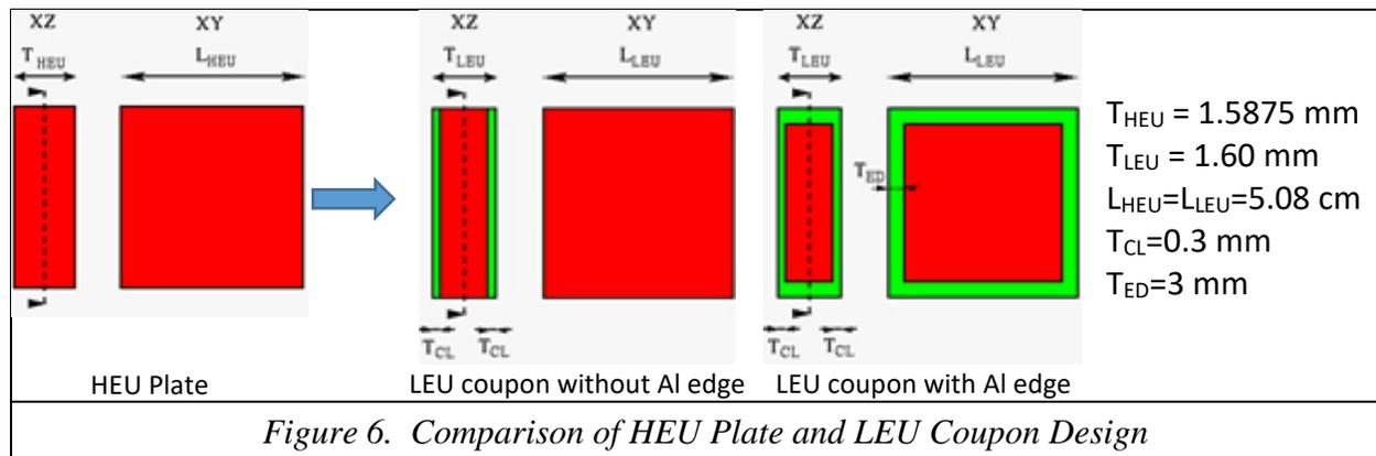
The coating or cladding material had to be as transparent as possible to neutrons in order to not affect the neutron spectrum of the assemblies in KUCA. Starting with surrogate (non-radioactive) materials a comprehensive test matrix investigated sixteen solutions to the cladding challenge, grouped into four categories: aluminum spray coating, epoxy coating, organic box and aluminum box. Figure 7 shows a summary display of the various techniques that were attempted.
