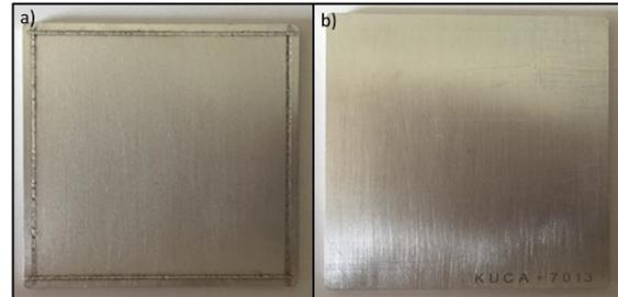
*Figure 9. Welded KUCA Dry Fuel Core Coupon*
