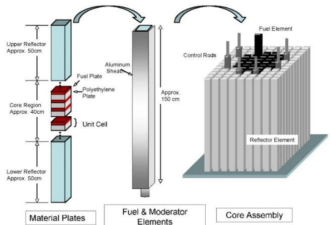
Figure 2. Schematic View of KUCA Dry Core Fuel Element and Assembly
