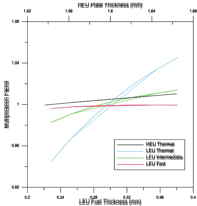
Figure 5. Sensitivity of Assembly  $k$ -eff to Fuel Thickness for Various Spectra
