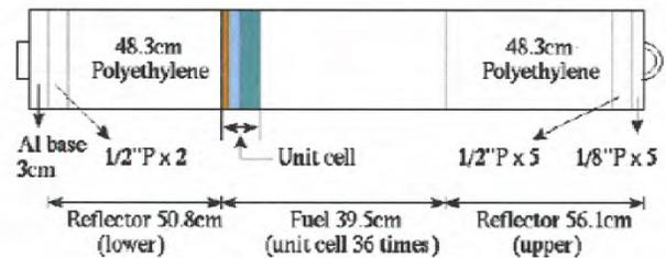
Figure 4. Cross Sectional View of KUCA Benchmark Assembly (A3/8"P36EU)
