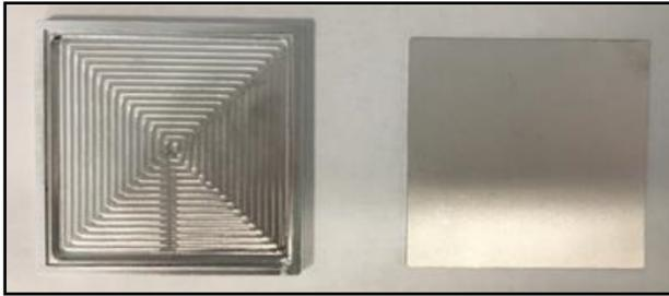
*Figure 8. Outer Box and Cover Plate Before Assembly*
