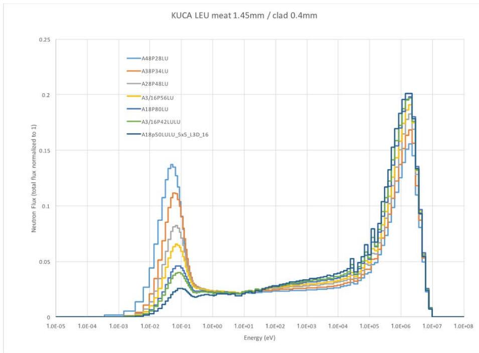
Figure 10. Neutron Spectra of Critical Cores of KUCA after LEU Conversion Using Thick LEU Coupon Design
