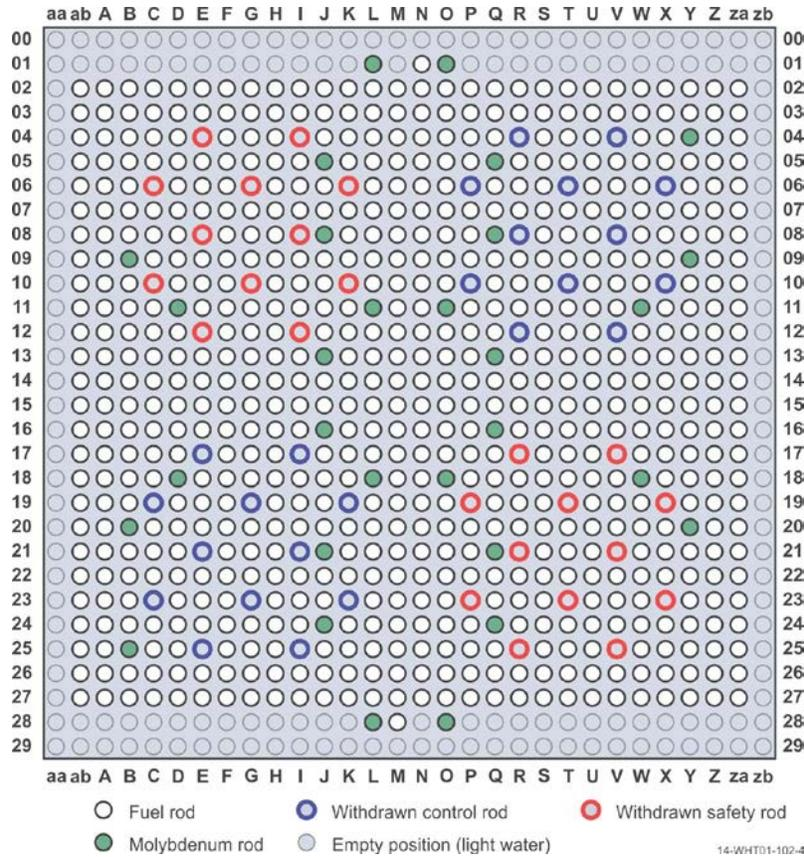
**Figure 3.** Core Configuration for the IPEN/MB-01 Reactor with 30 Molybdenum Rods [9].
