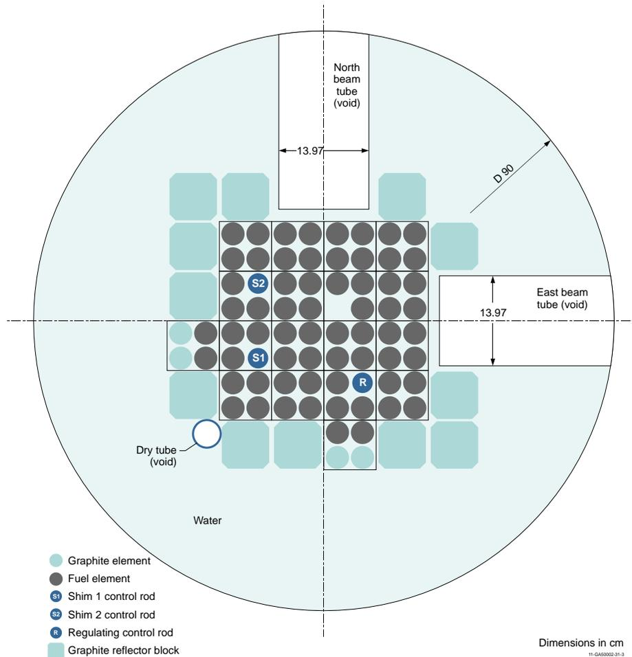
**Figure 2.** NRAD Benchmark Model Mid-Plane Cross Section (64 Fuel Element Loading) [8].
