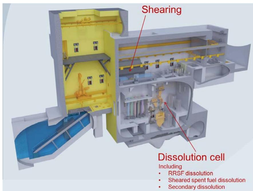
Fig. 5: Overview of main TCP facility operations
