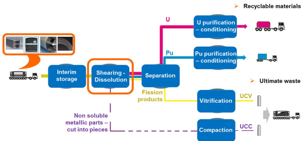
Fig. 4: Process diagram for RRSF reprocessing on La Hague site
