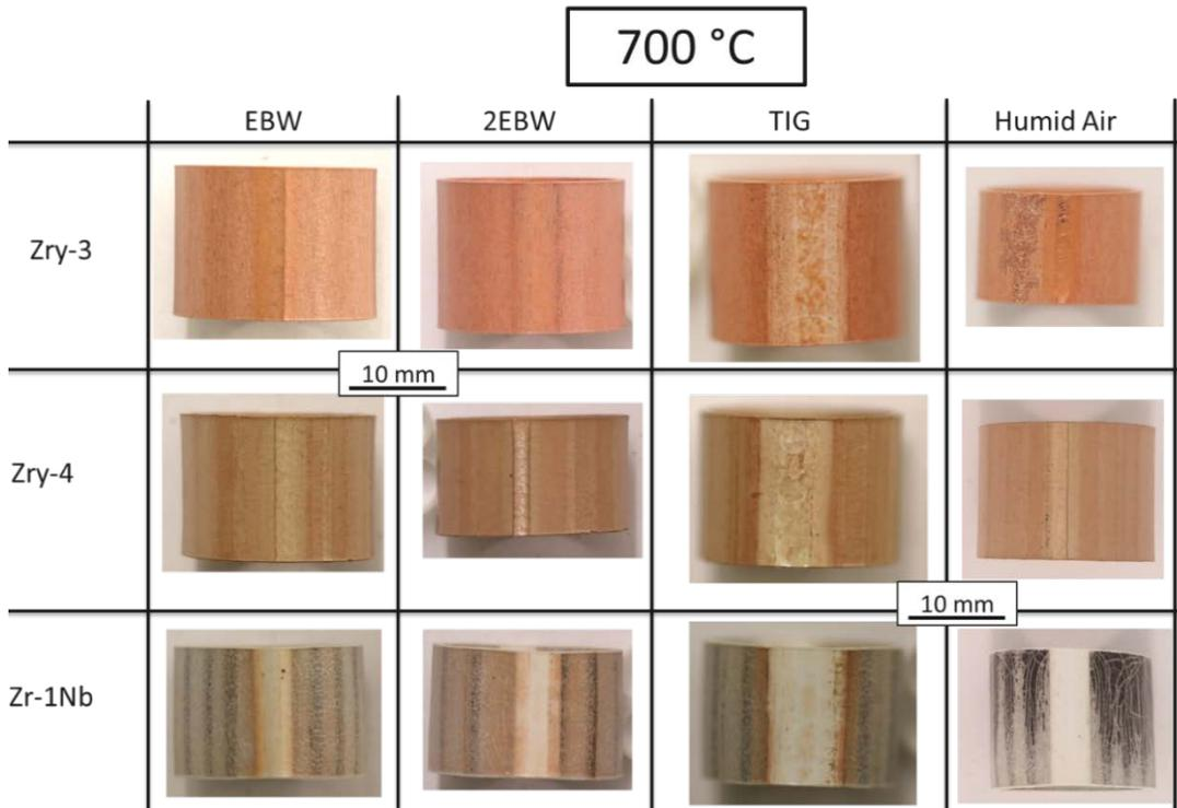
**Figure 7: Oxidation on weld affected areas and humid air**
