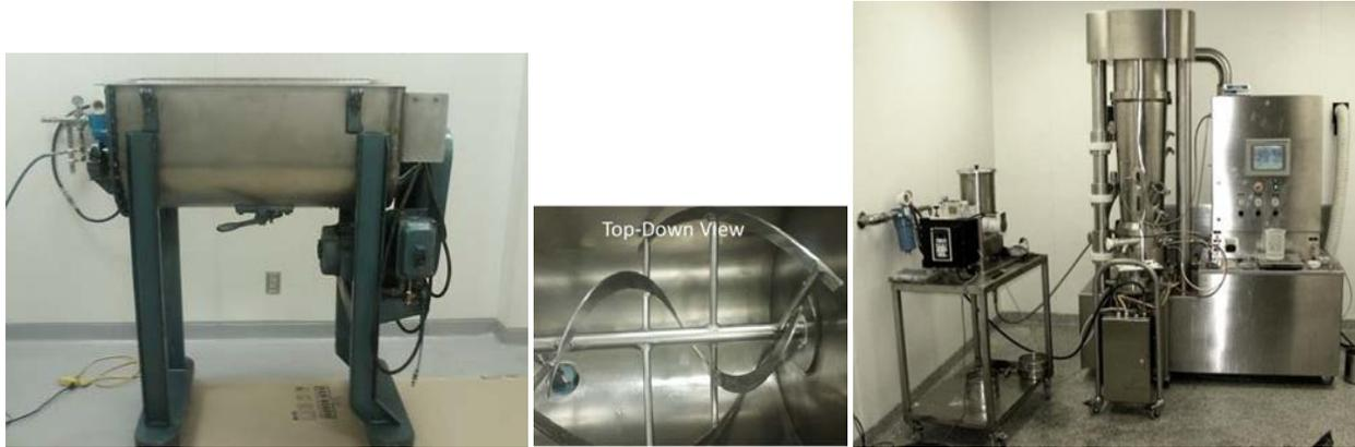
**Figure 3: Left – ribbon blender; center – inside ribbon blender; right – granulator**
