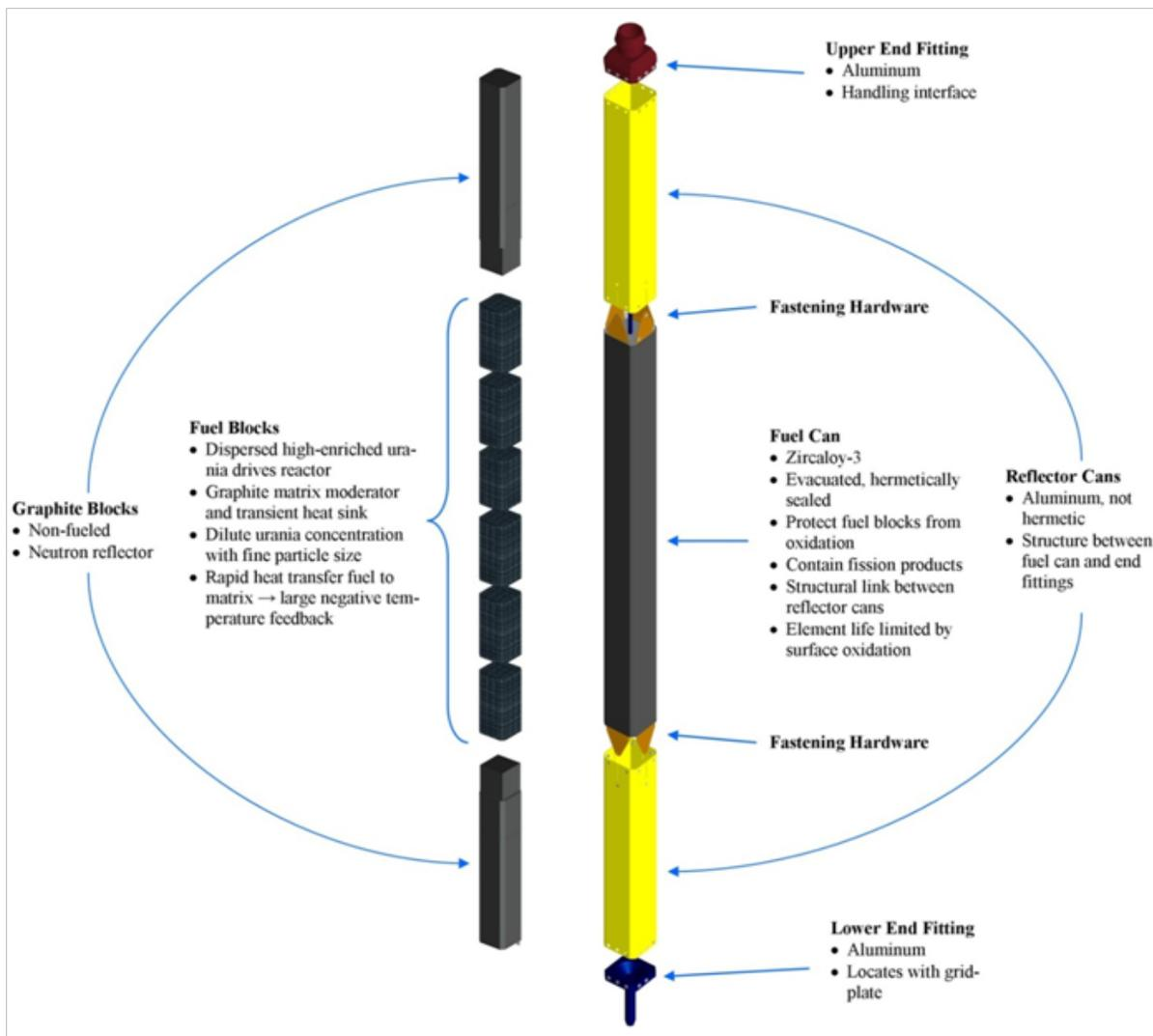
Figure 1. Assembly schematic for existing TREAT fuel elements.
