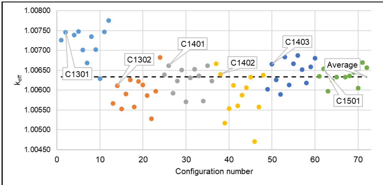
**Figure 2-3 MCNP  $k_{ECP}$  Values After Moderator Temperature Correction**
