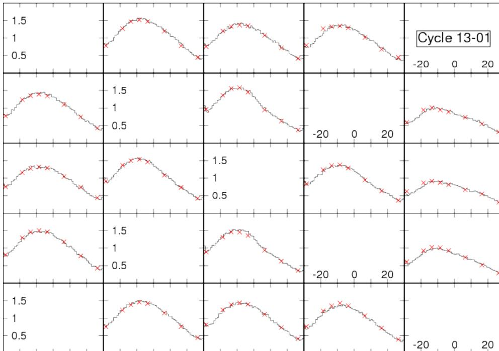
**Figure 2-4 Calculated (black line) and measured (red crosses) results for Cu foil activation in cycle 1301, in relative units**
