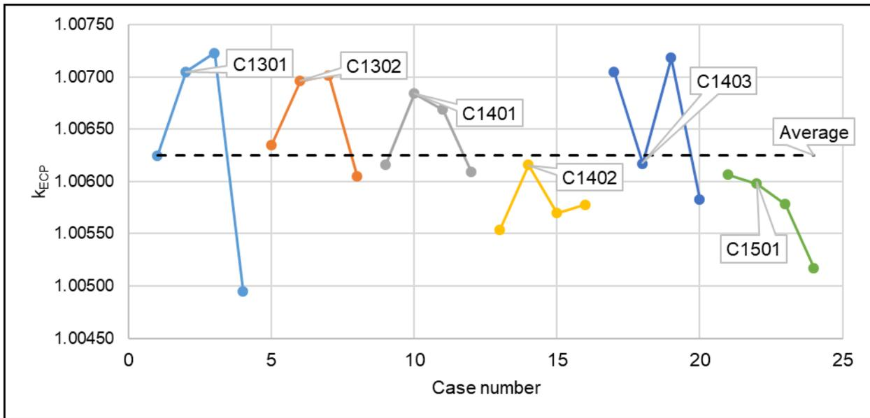
**Figure 2-1 Moderator Temperature Corrected MCNP  $k_{ECP}$  Values for Validation Cases**
