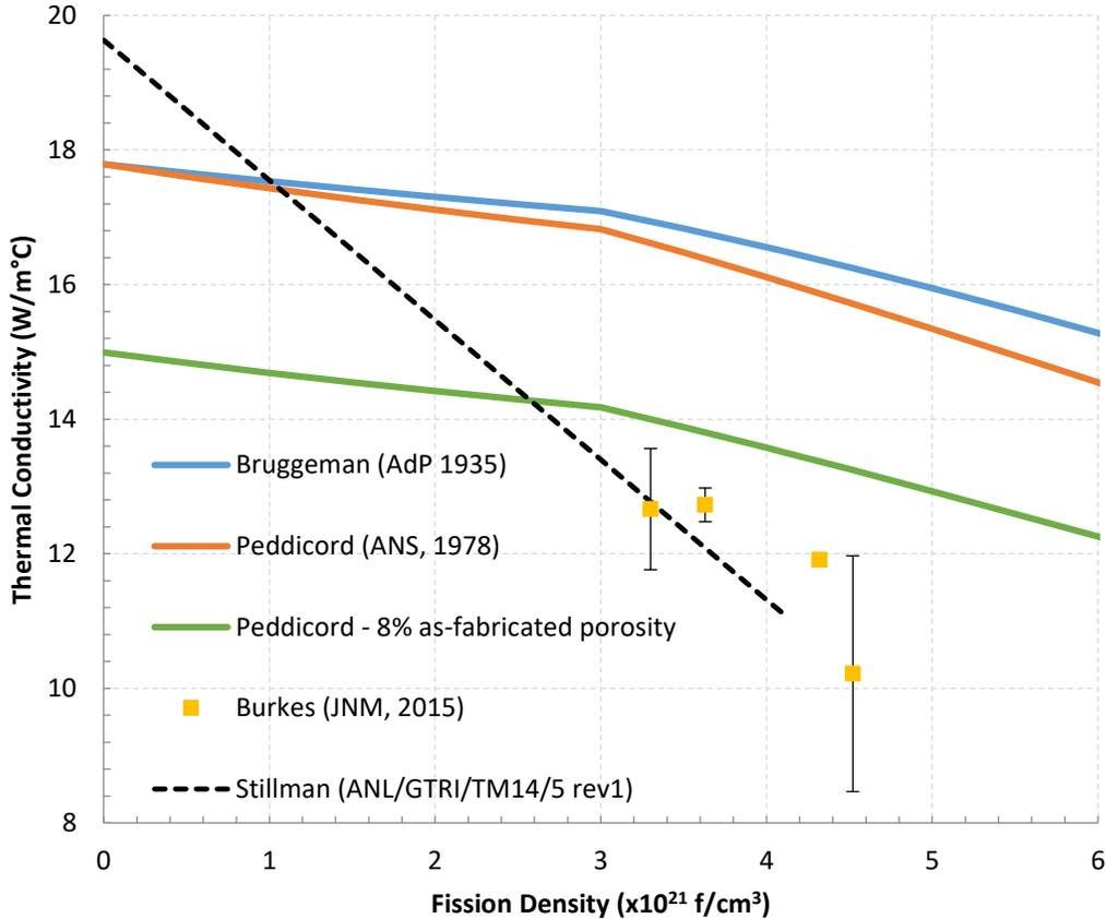
Figure 5: Thermal conductivity of U-10Mo fuel radiation dependence, 8% as-fabricated porosity addition to Peddicord model
