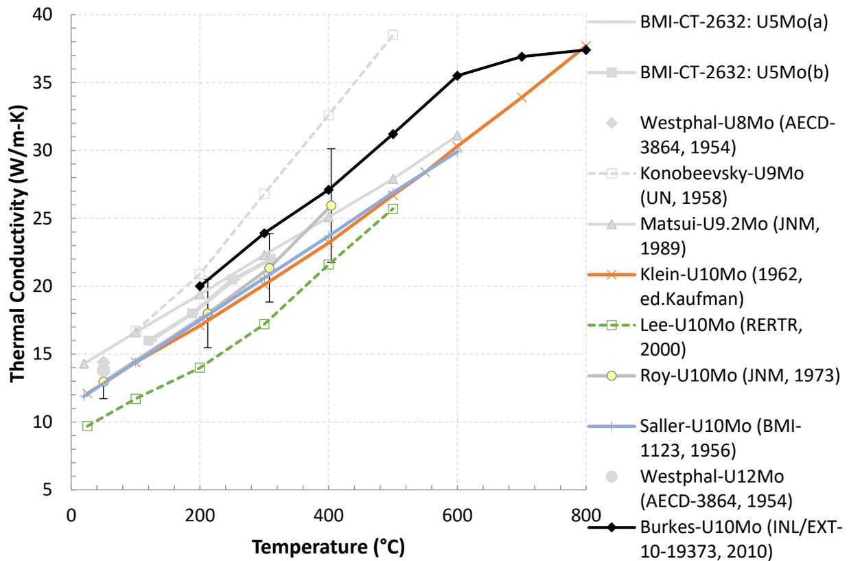
Figure 3: Thermal conductivity of U-Mo alloys temperature dependence
