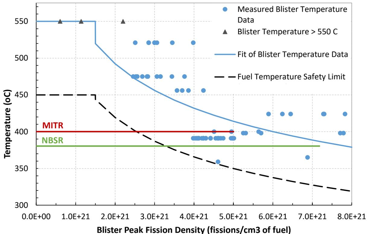
Figure 6: Blister temperature of U-Mo fuel plates with irradiation
