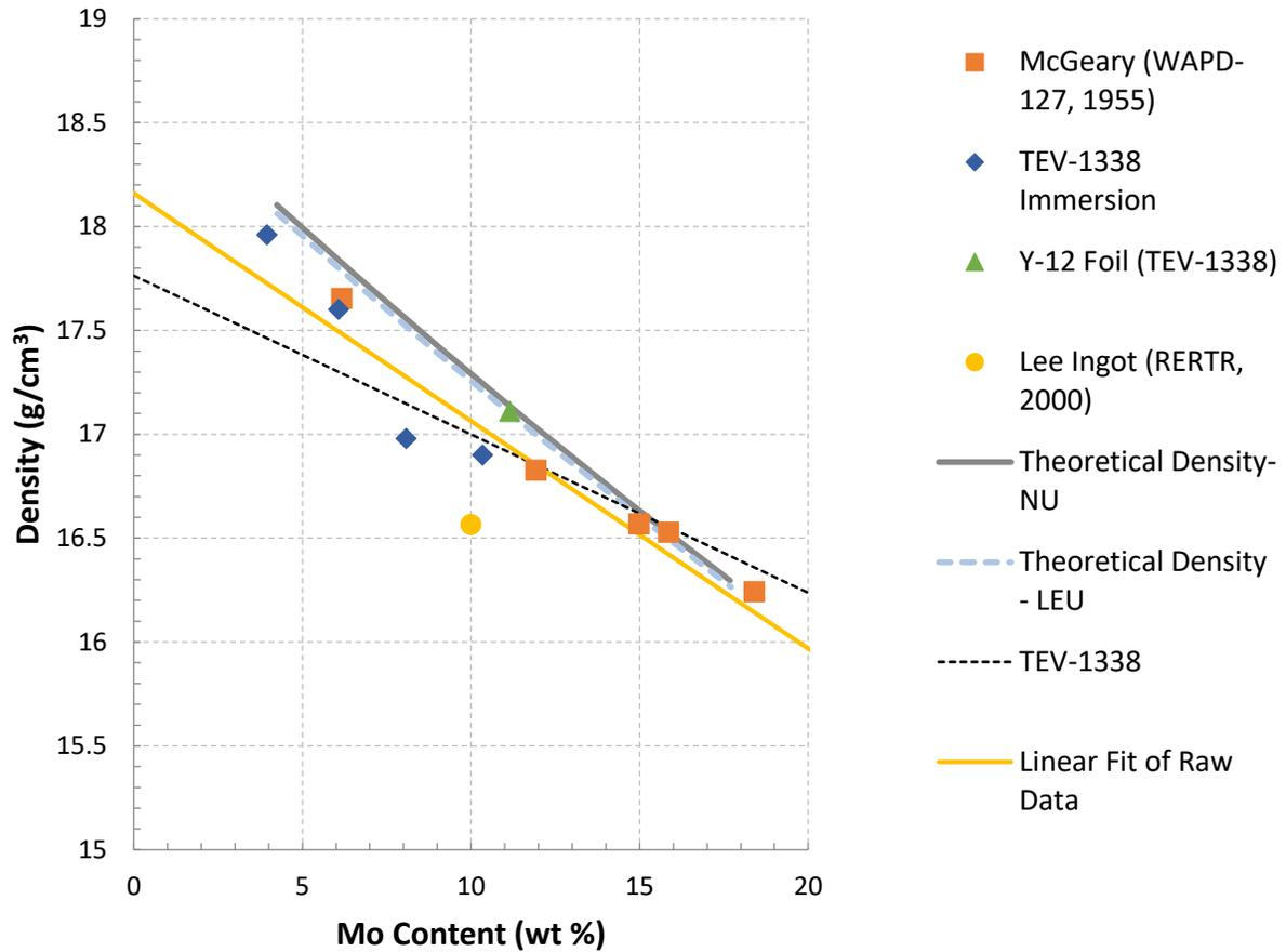
Figure 1: Dependence of the density of U-Mo alloys on Mo content.
