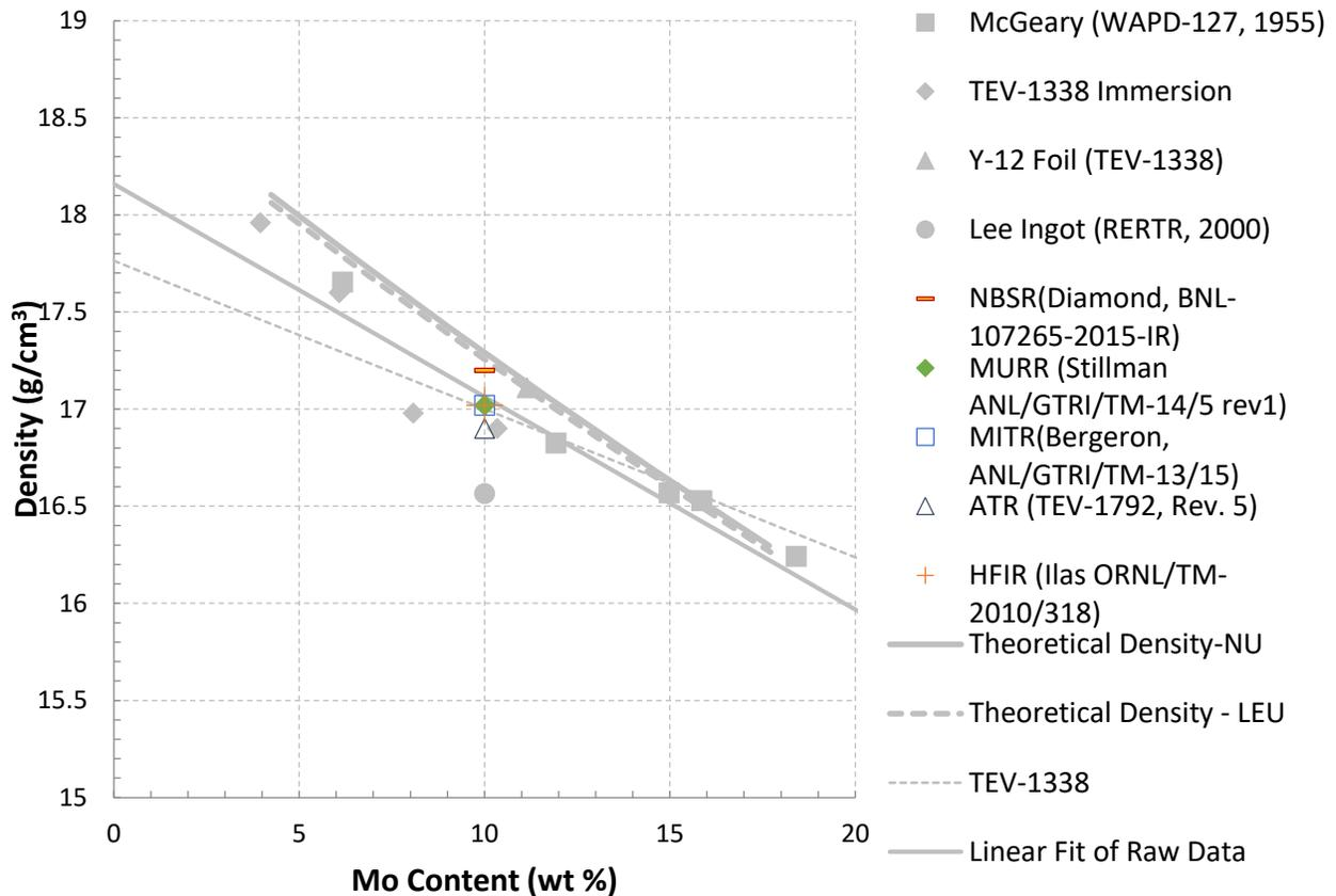
Figure 2: Comparison of U-10Mo density assumptions of the USHPRR with the experimental data.
