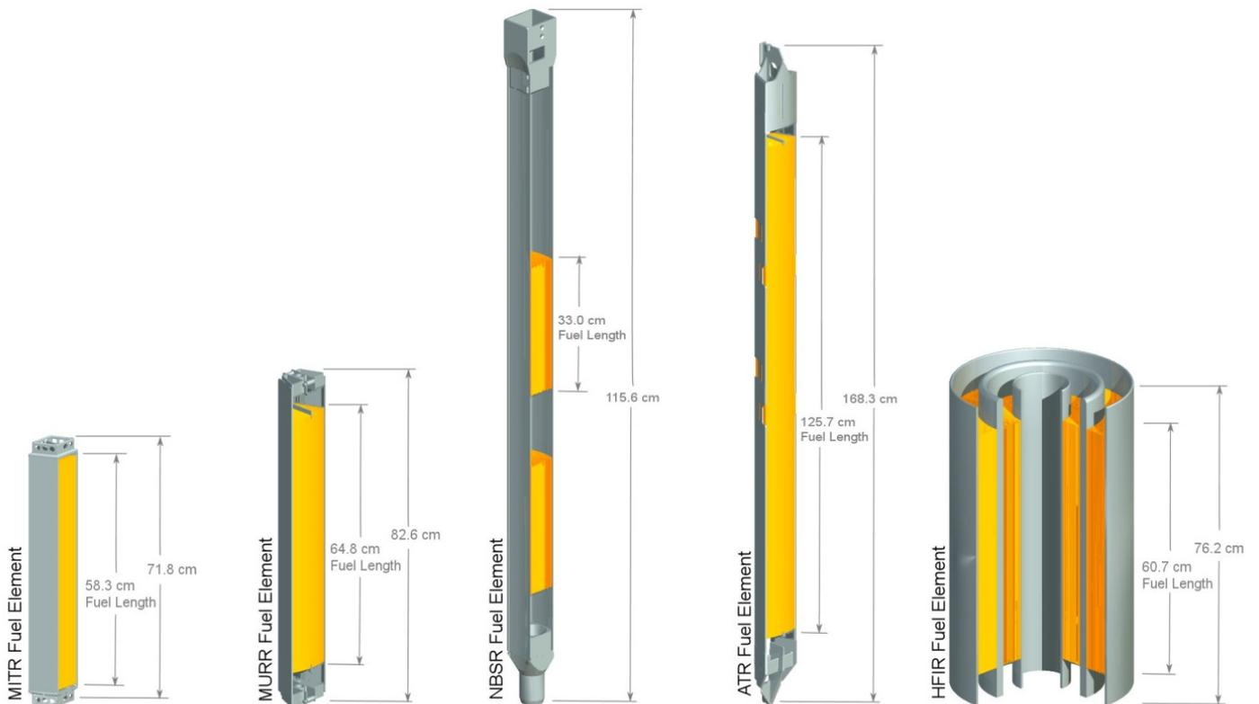
Figure 4: HPRR Fuel Assembly Designs, Isometric Views
