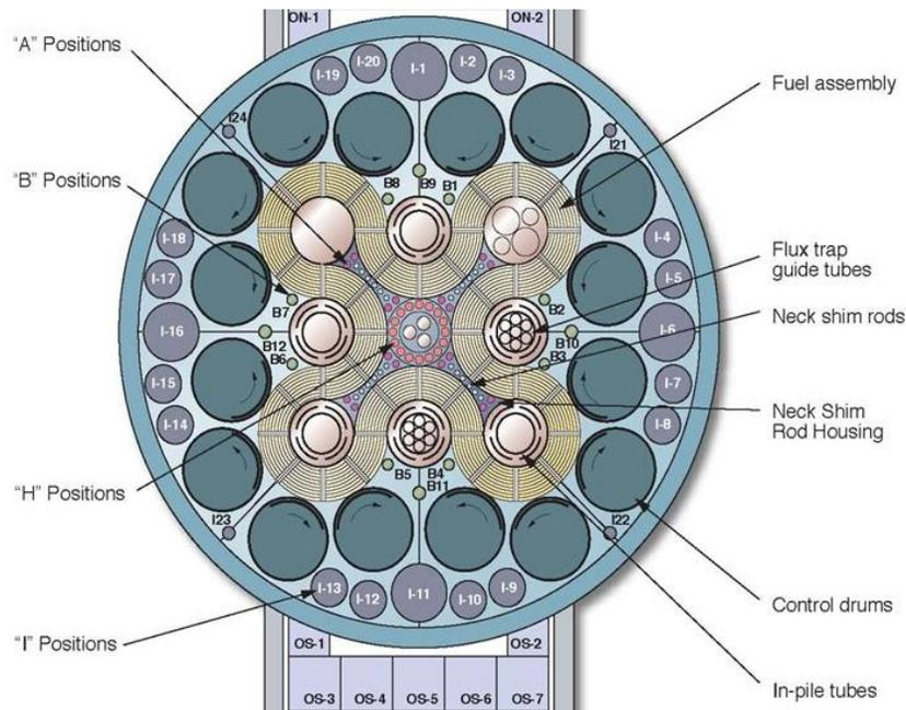
Figure 6: ATR Core Map Illustrating Driver Fuel, Flux Trap, and Reflector Positions
