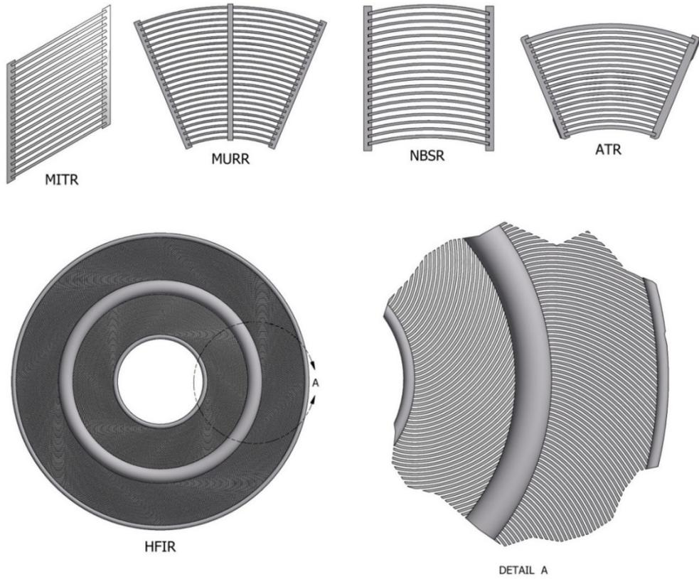
Figure 3: HPRR Fuel Assembly Designs, Top Views
