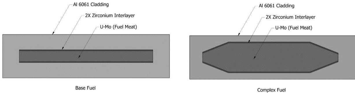
Figure 1: Cross Section of Fuel Designs
