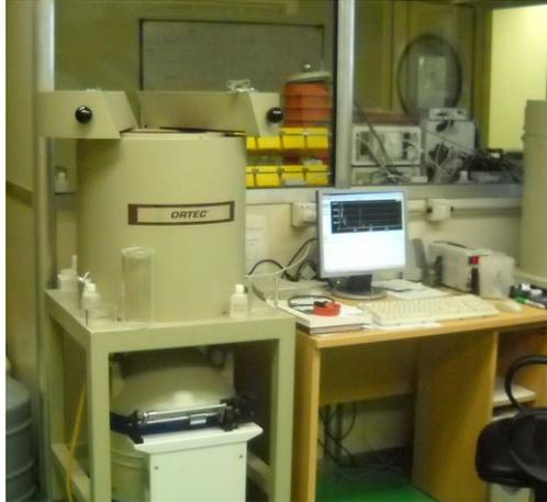
Fig. 2. HPGe detector used in the measurement of filters post-dissolution.
