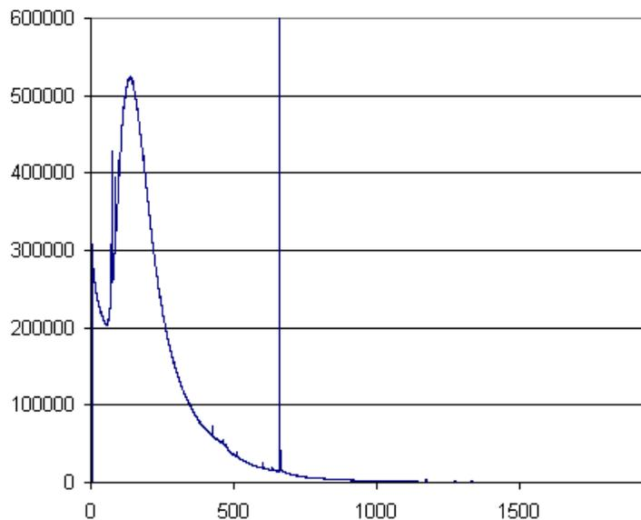
Fig. 1. Spectrum obtained with Genie-2000 using a HPGe detector. The data obtained was transferred to a spreadsheet in order to be able to analyze it.
