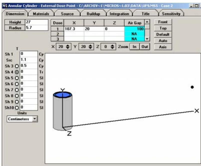
Fig. 4. Microshield chase. A cylinder including the source distributed in it was used as model.
