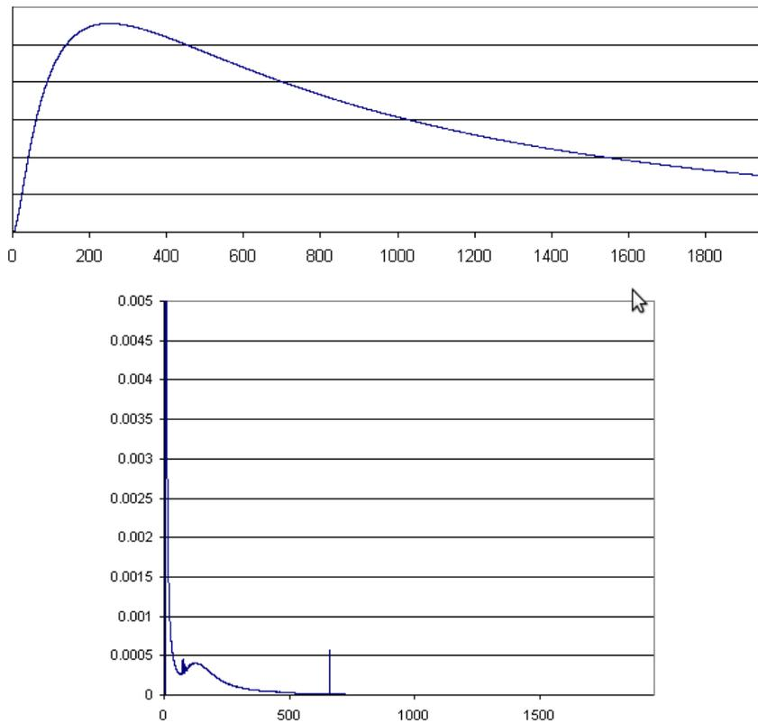
Fig. 3. Relative efficiencies obtained from the peaks of Sb-125 and efficiency-independent emission spectrum. It can be viewed the relative importance of low energy emission due to bremsstrahlung of beta emitters interacting with the wall of the container cartridge.
