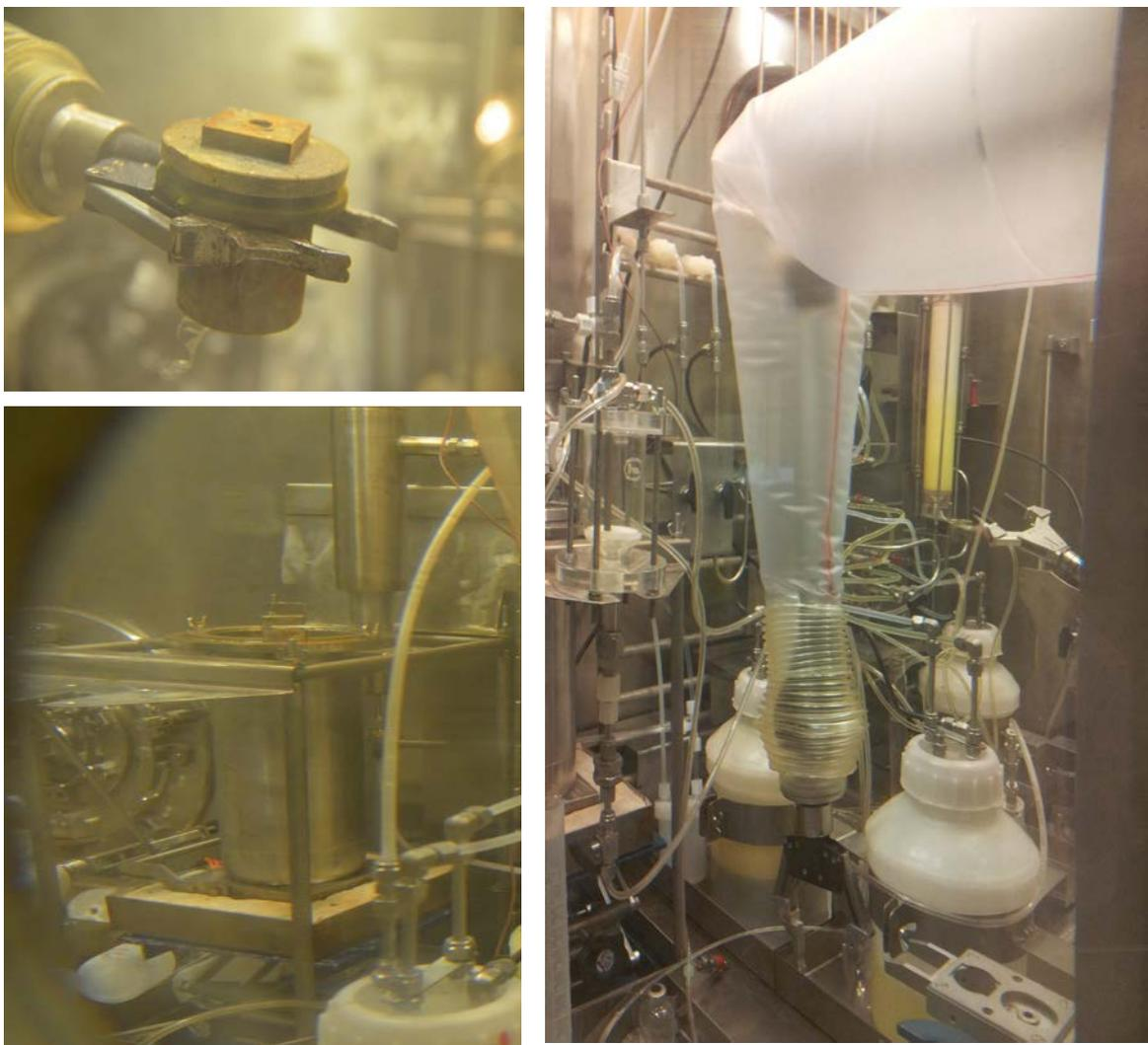
Figure 2 – Top left a filter with its lid, bottom left the dissolver and on the right an overview of the hot cell extraction chromatographic purification process.
