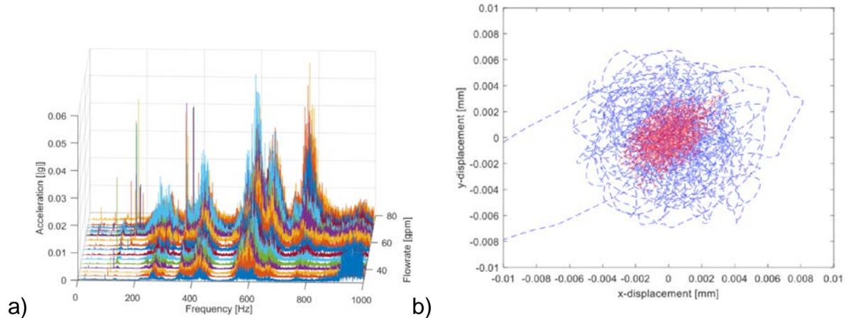
**Figure 10. a) Frequency content of the Large B experiment motion as a function of flow rate, b) integrated position path cloud for basket (blue) and simulator (red)**
