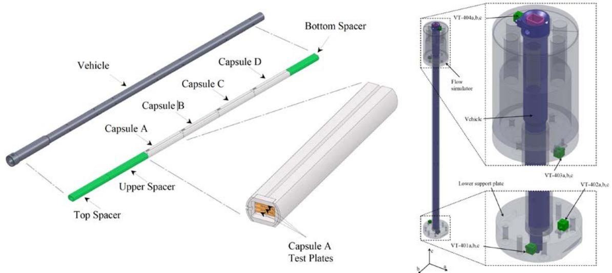
**Figure 2. MP-1 Large B Experiment and Position Simulator**
