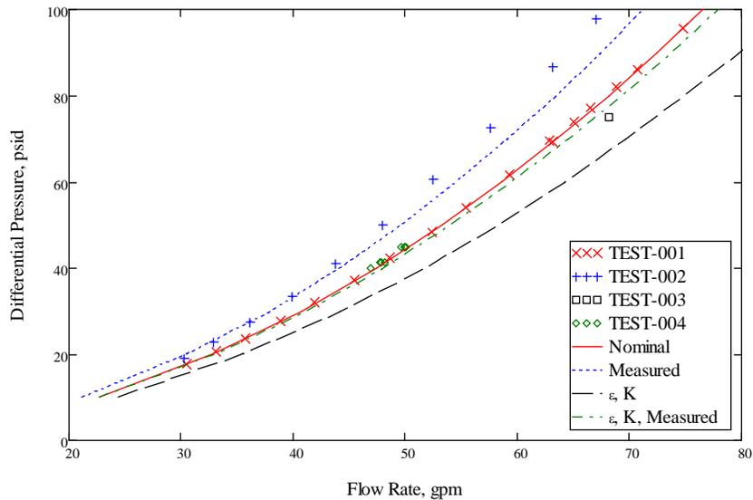
**Figure 7. HMFTF Test Data comparison with 'tuned' RELAP5 models.**
