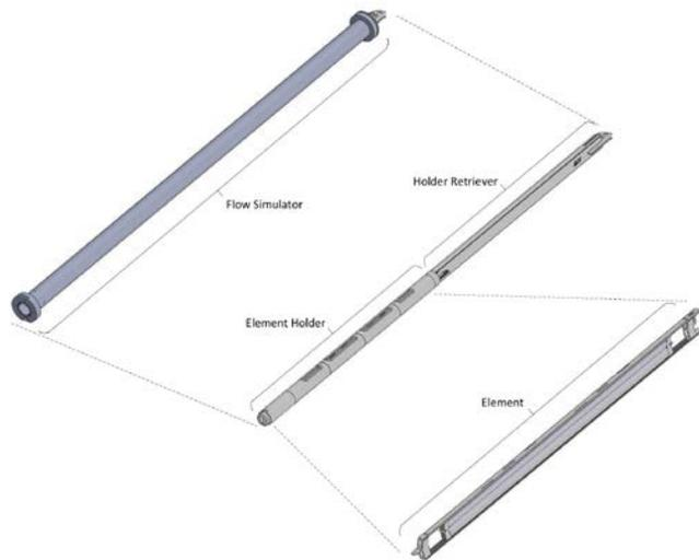
**Figure 6. AFIP-7 flow test hardware**
