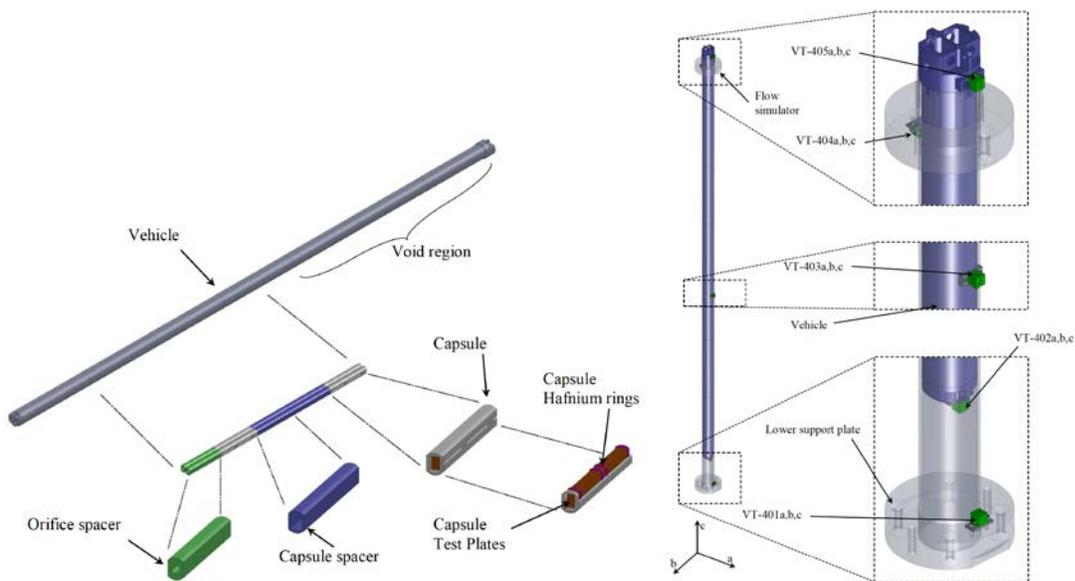
**Figure 3. MP-1 High Power Experiment and CDIPT position simulator**
