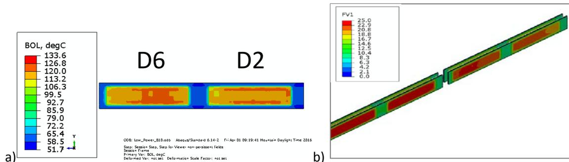
**Figure 8. a) Beginning of Life fuel centerline temperature, select plates in Low Power B-10 capsules, b) End of Life Oxide Thickness (microns), select plates in Low Power B-10**
