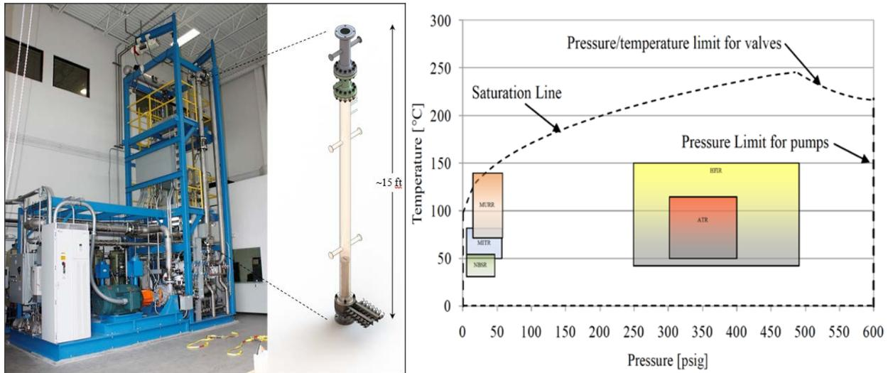
**Figure 1. HMFTF and its design envelope with HPRR operational envelopes**
