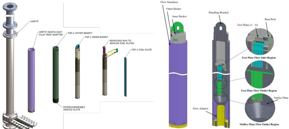
**Figure 5. FSP-1 flow test hardware**
