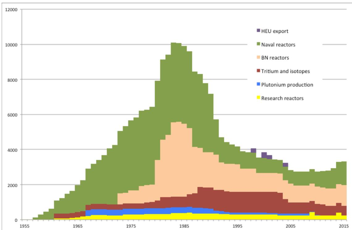
Figure 1. Estimated consumption of HEU as fuel in the Soviet Union and Russia, kg of 90% HEU equivalent.
