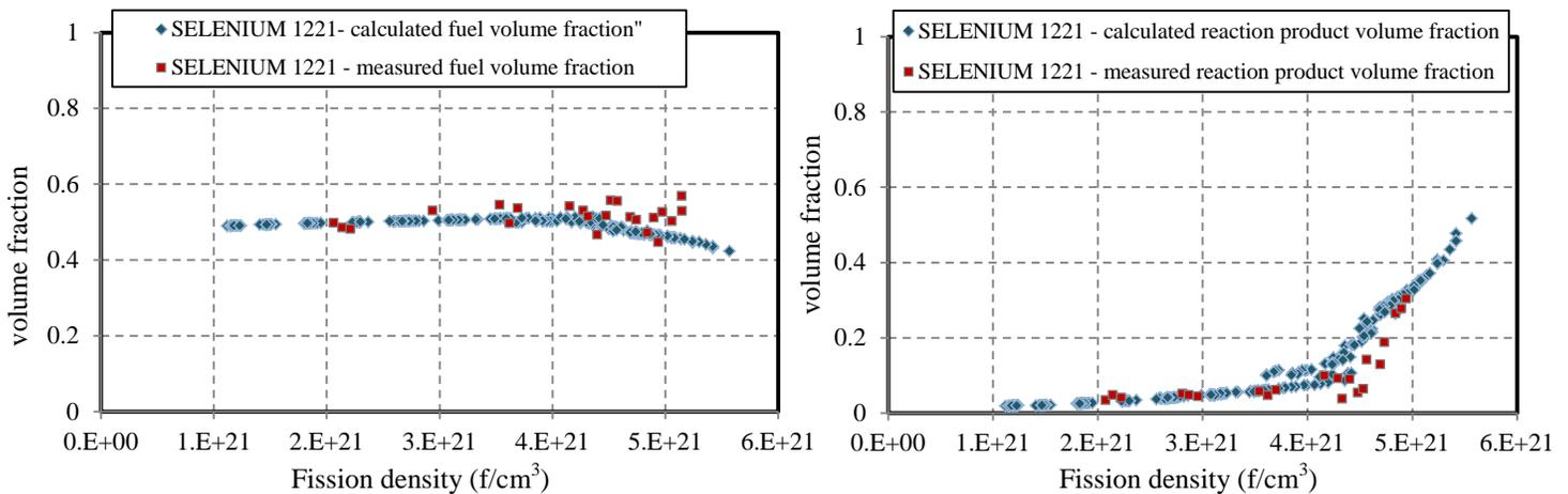
Fig. 4 Calculated fuel and IL volume fractions in the SELENIUM U7MD1221 plate, compared to experimental data [21].
