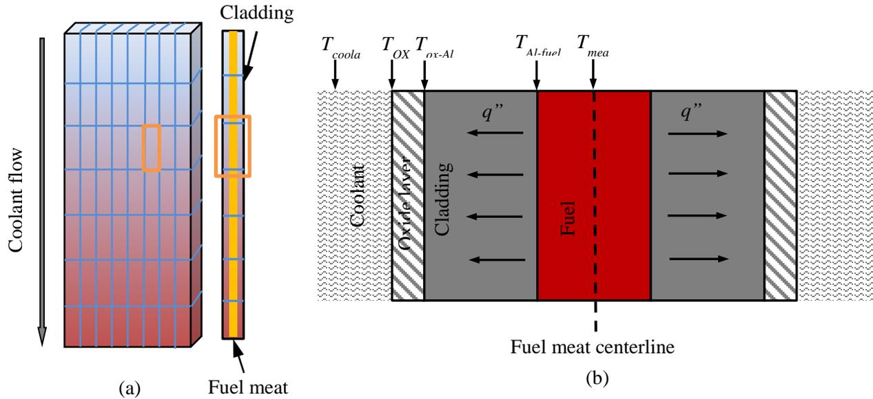
Fig.2 (a) An example of the meshing scheme in the DART-2D framework, and (b) enlarged side view of one fuel plate node indicated in (a) and schematic representation of the temperatures calculated to obtain fuel meat centerline temperatures.
