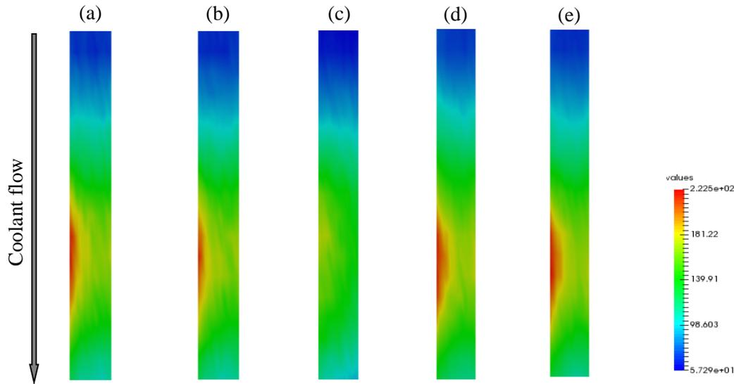
Fig. 10 Representative fuel meat centerline temperature distributions in (a) the SELENIUM 1221 plate, (b) the SELENIUM 1231 plate, (c) the SELENIUM-1a plate, (d) the E-FUTURE 4202 plate, and (e) the E-FUTURE 6301 plate.
