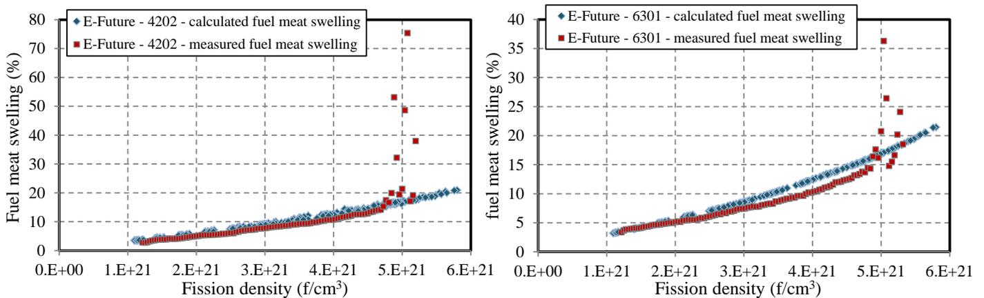
Fig. 7 A comparison of calculated and measured fuel meat swelling of the E-FUTURE U7MC4202 and U7MC6301 plates [17].
