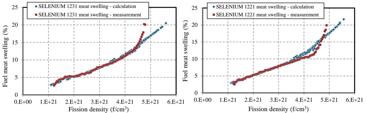
Fig. 5 Comparisons of calculated and measured fuel meat swelling [4] of the SELENIUM U7MD1231 and U7MD1221 plates.
