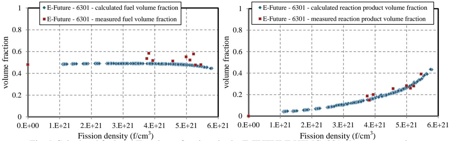
Fig. 9 Calculated fuel and IL volume fractions in the E-FUTURE U7MC6301 plate, compared to experimental data [22].
