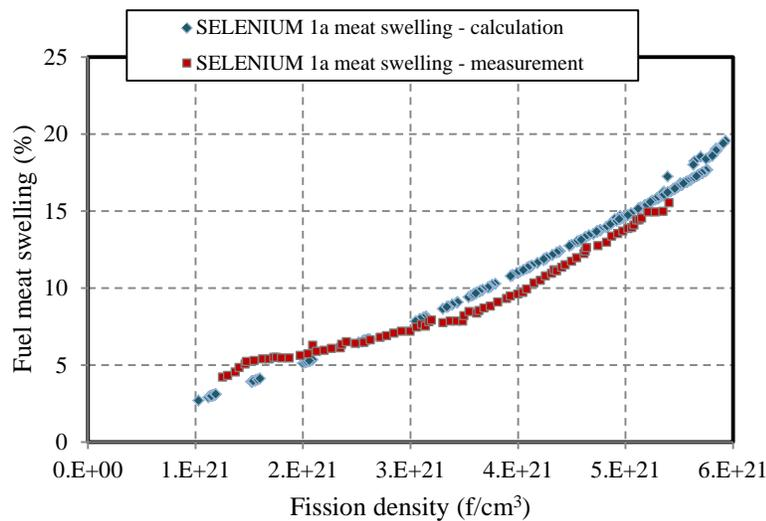
Fig. 6 A comparison of calculated and measured fuel meat swelling of the SELENIUM-1a plate.
