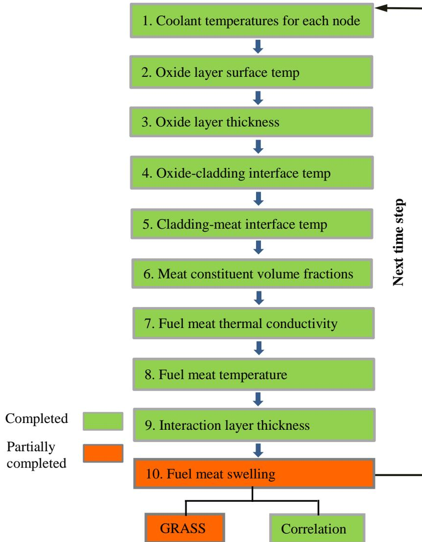
Fig. 1 Flow chart of the DART-2D framework. Different color indicates the current completion status of each function.
