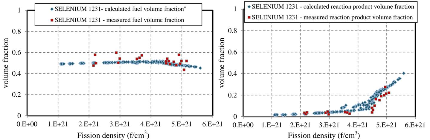
Fig. 3 Calculated fuel and IL volume fractions in the SELENIUM U7MD1231 plate, compared to experimental data [21].
