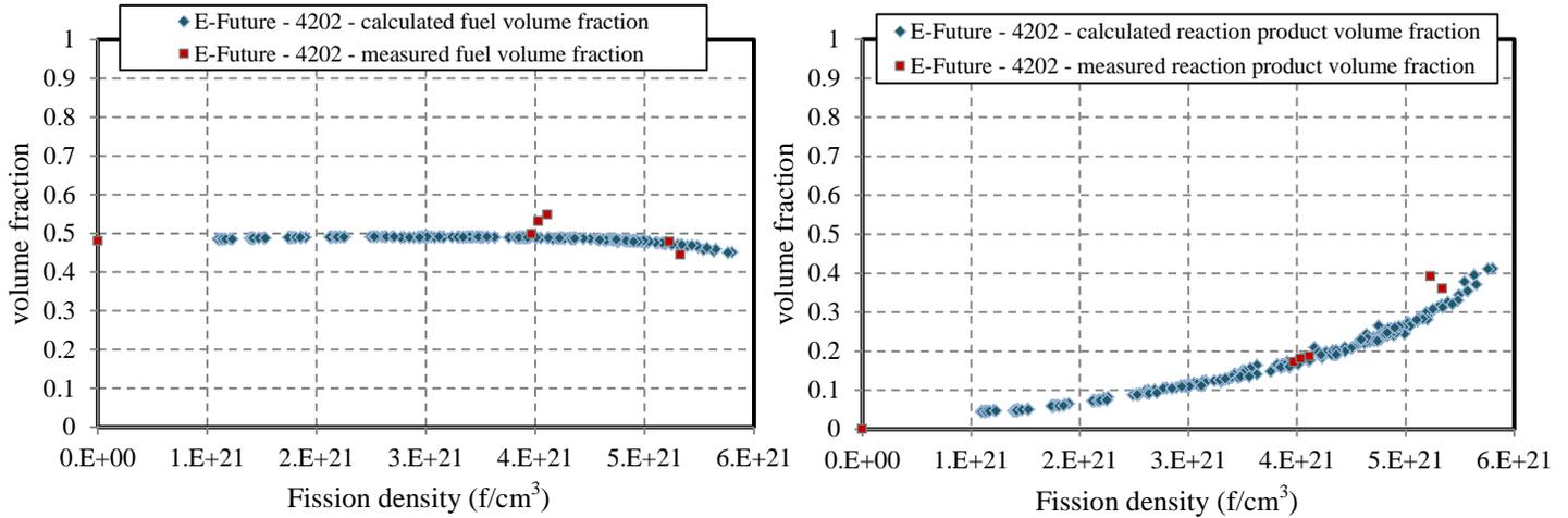
Fig. 8 Calculated fuel and IL volume fractions in the E-FUTURE U7MC4202 plate, compared to experimental data [22].
