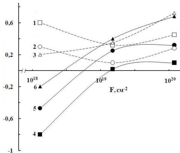
Fig. 1. The relative change in linear dimensions of the samples of aluminum alloys having the shape of a parallelepiped (1 and 4), a cylinder (2, 5) and drive (3, 6) depending on the fast neutron fluence. The solid line shows the variation along the long side of the samples (4-6), the dashed - thickness of samples (1-3).
