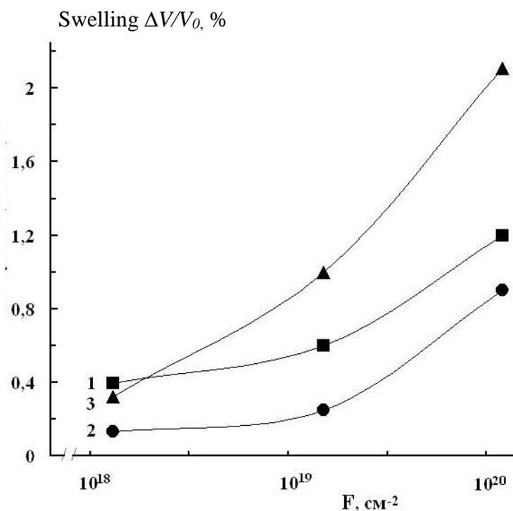
Fig. 2. Relative change in volume of the samples of aluminum alloy 96,8Al + 2,4% Mg + 0,3% Cu, having a parallelepiped shape (1), a cylinder (2) and the disc (3) according to the fast neutron fluence.
