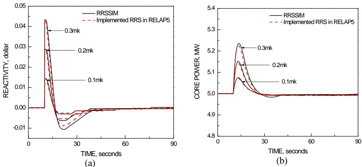
**Figure 4 Comparisons of reactivity and power in the ramp insertions of reactivity (Reactivity (a), Core power (b))**
