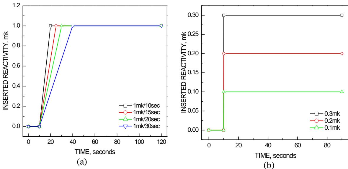
**Figure 2 Reactivity insertion rates for ramp insertion (a) and step insertion (b)**
