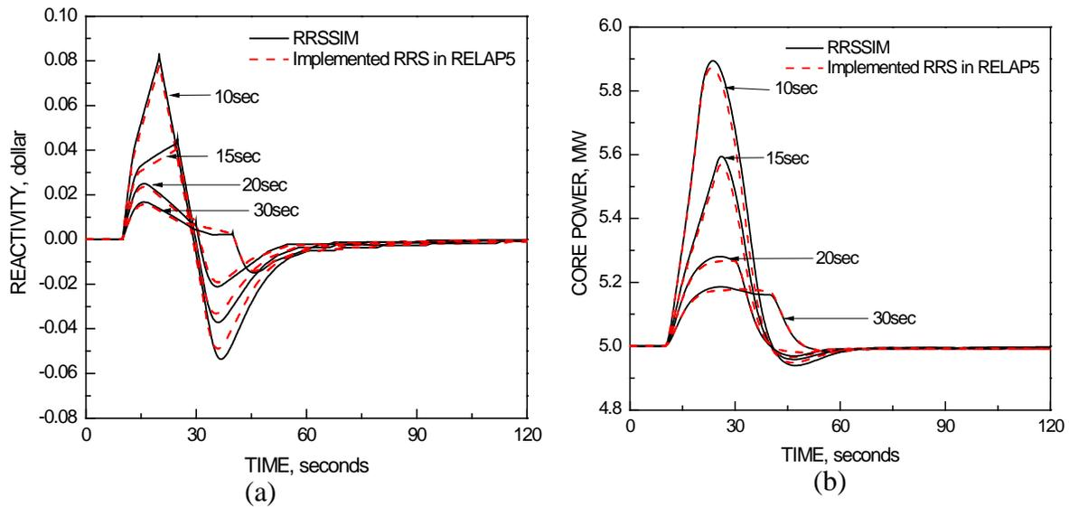
**Figure 3 Comparisons of reactivity and power in the ramp insertions of reactivity (Reactivity (a), Core power (b))**
