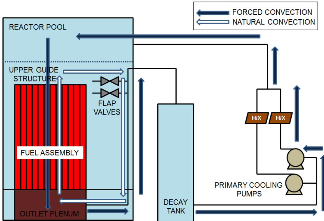
**Figure 5 Schematic diagram of forced convection and natural convection mode**
