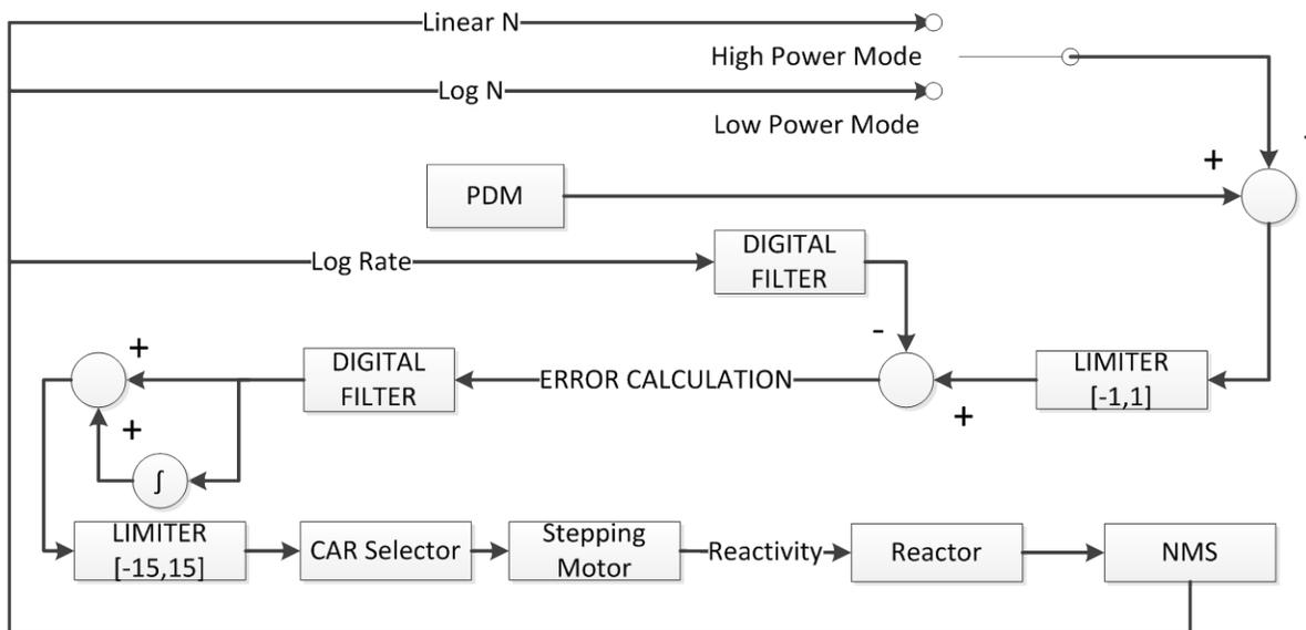
**Figure 1 Reactor power control algorithm**
