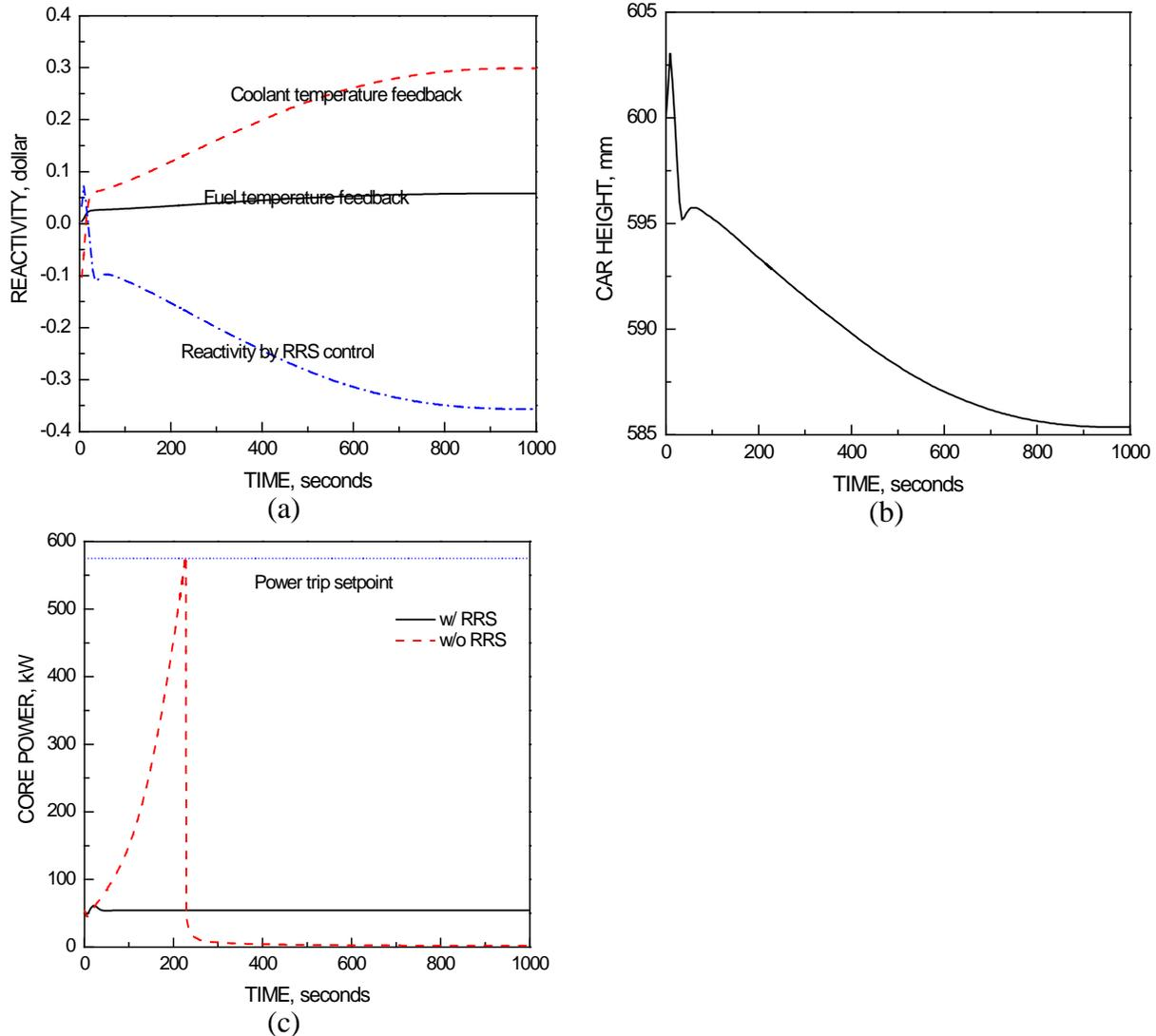
**Figure 6 Results of cold water insertion accident with respect to RRS action**
