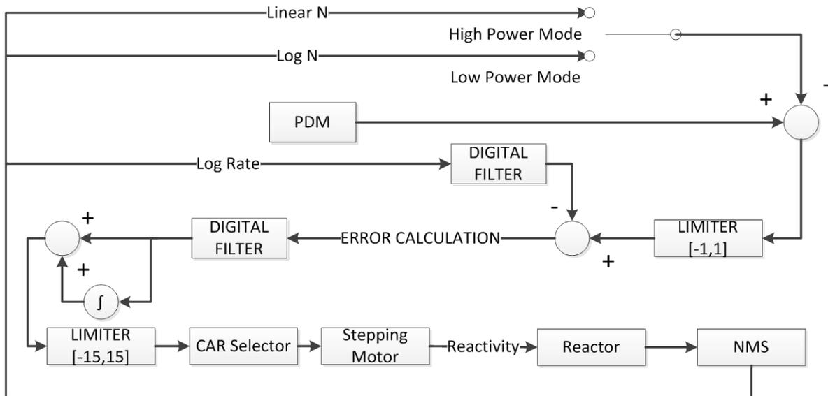
**Figure 1 Reactor power control algorithm**
