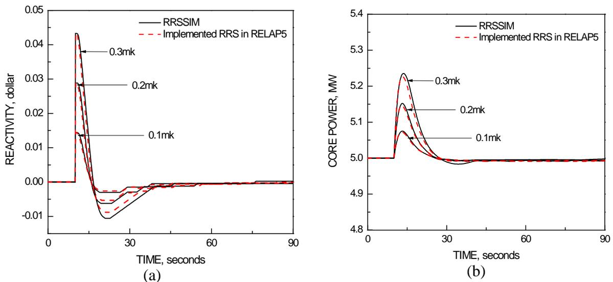
**Figure 4 Comparisons of reactivity and power in the ramp insertions of reactivity (Reactivity (a), Core power (b))**
