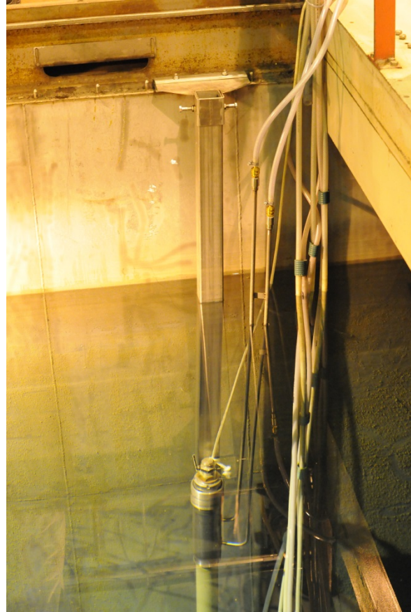
Figure 5 Side view of measuring stand with channel with spent fuel element inserted.
