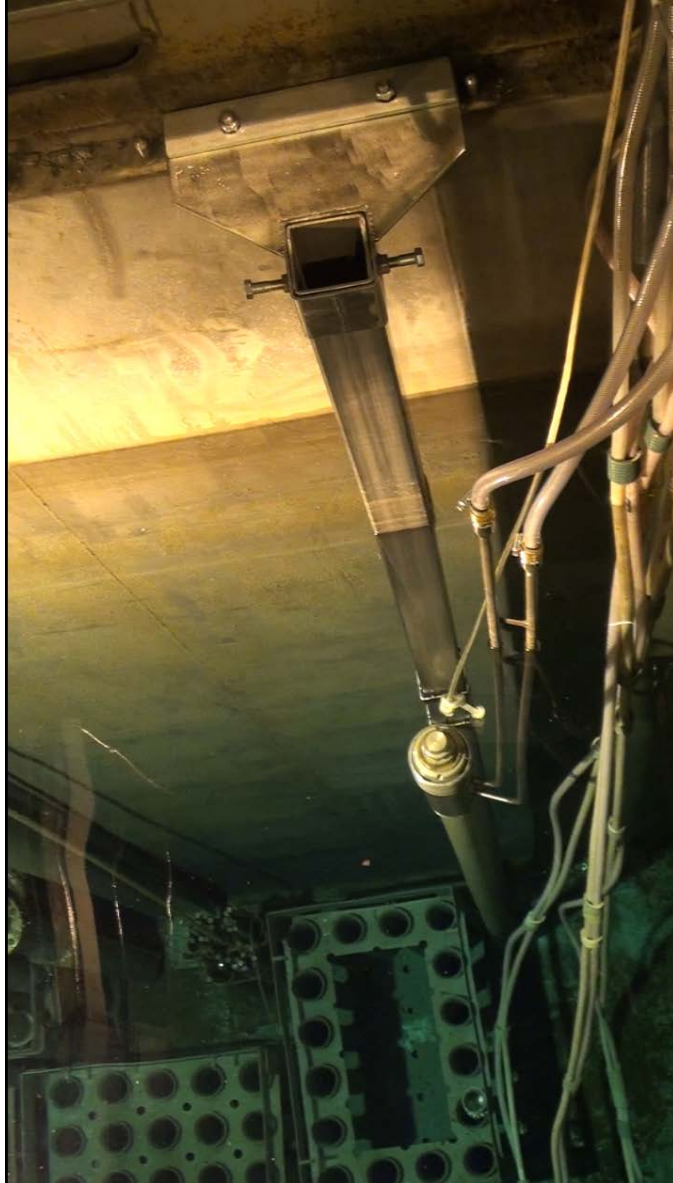
Figure 4 Top view of measuring stand with channel with spent fuel element inserted.
