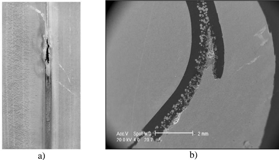
Figure 9. Fuel element with a defect (a) and cross-cut at the place of defect (b).
