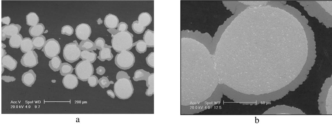
Figure 4. SEM images of macro- and micro-structure of IRT-3M No.2 FA fuel meats.
