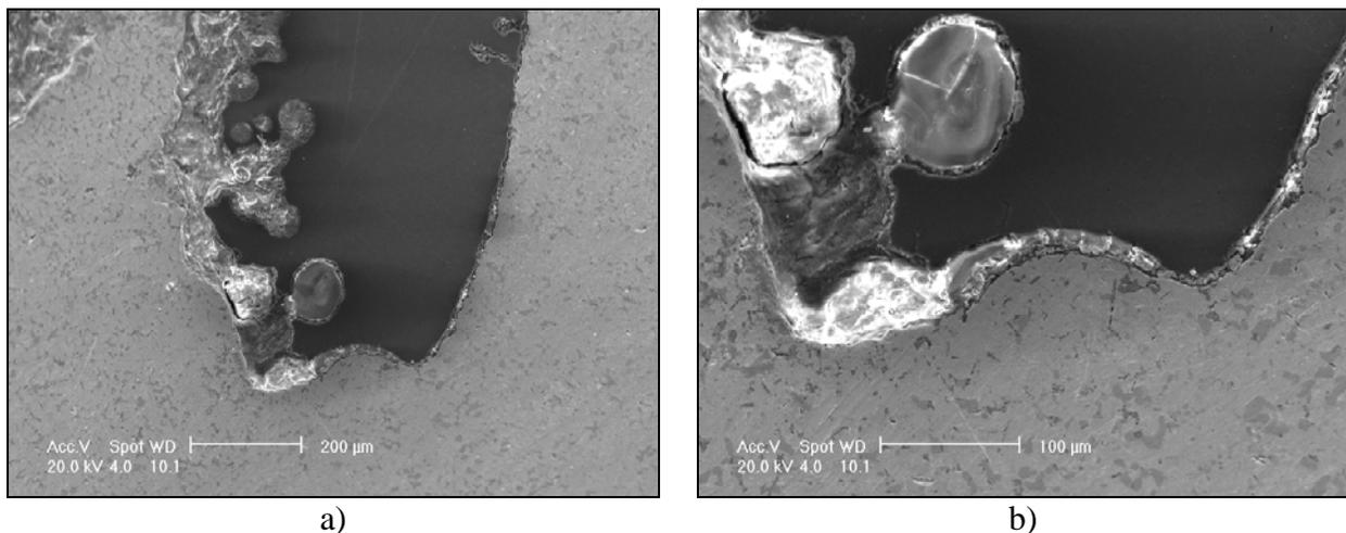
Figure 10. Micro-structure of the fuel meat at the place of defect. The area marked on the left-hand photo is zoomed on the right-hand one.
