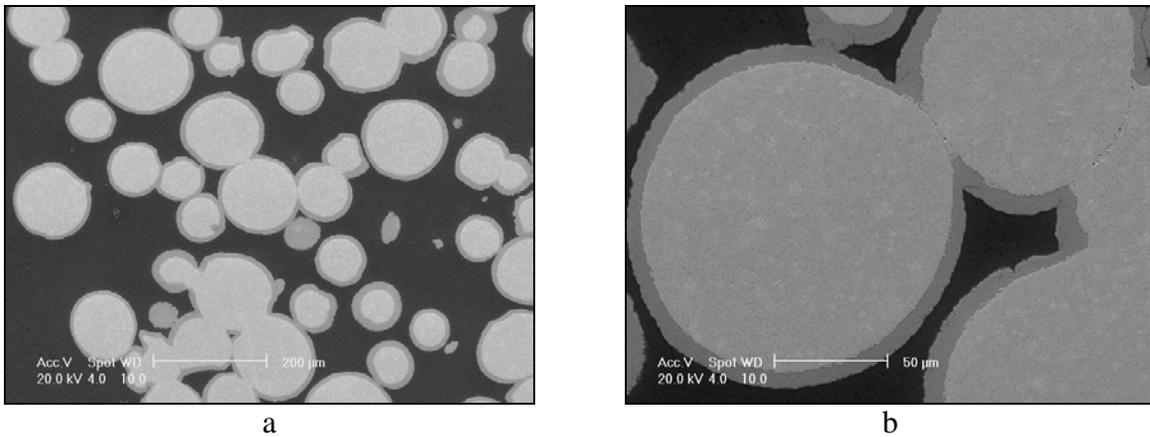
Figure 5. SEM images of macro- and micro-structure of IRT-U No.2 FA fuel meats.
