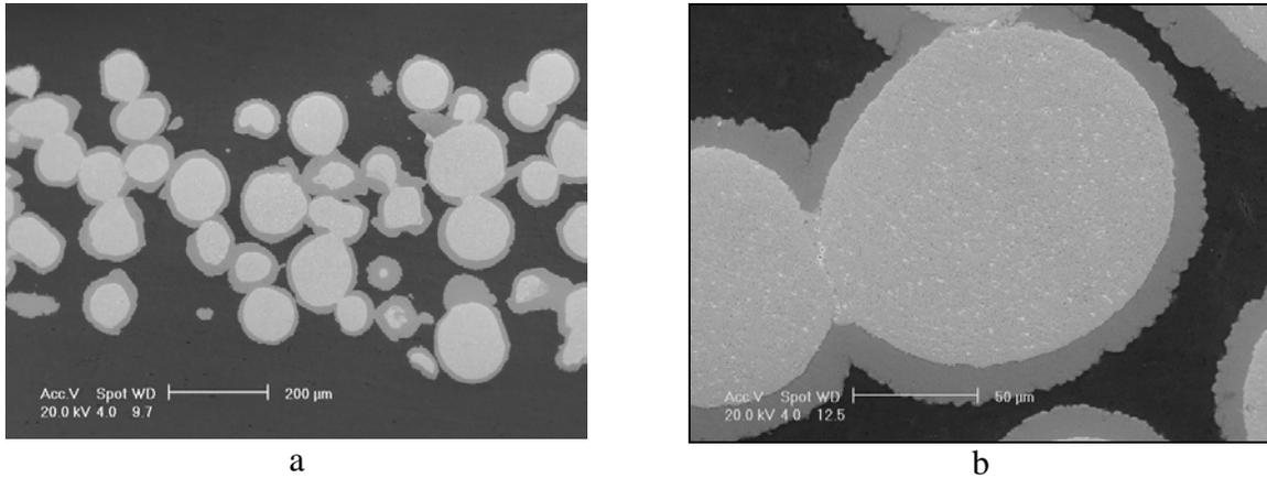
Figure 4. SEM images of macro- and micro-structure of IRT-3M No.2 FA fuel meats.
