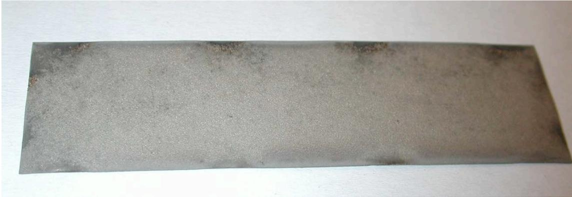
Fig. 6. Surface of Zr coated SS sample sprayed using the tapered head screws.
