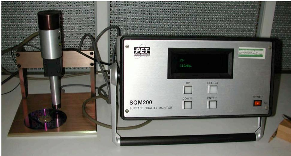
Fig. 1. Photoelectron measurement instrument with the UV source and electron detector on the left side of the image above the grounded sample holding surface.
