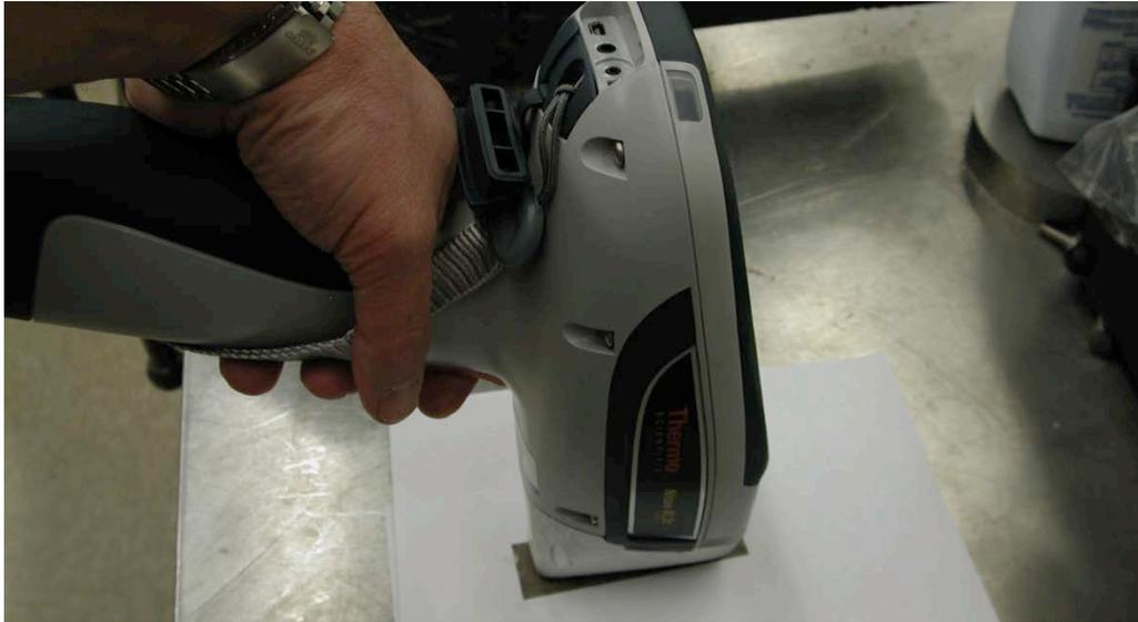
Fig. 3. Handheld XRF instrument measuring the Zr thickness of a coated sample.
