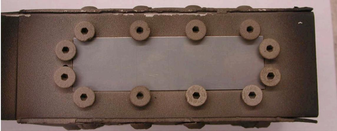
Fig. 2. Sample mounted in square tube using tapered head screws prior to Zr plasma spraying.
