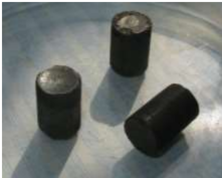
Figure 2 – Raw material – \text{UO}_2 with enrichment 1.8% and prepared solution of uranyl sulphate
