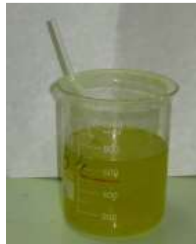
Figure 2 – Raw material – \text{UO}_2 with enrichment 1.8% and prepared solution of uranyl sulphate
