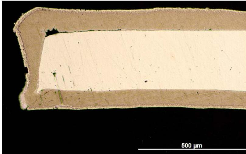
Fig. 12. Optical metallographic cross section of a stainless steel foil (center lighter object) with an 80  $\mu\text{m}$  Zr foil resistance welded to the top, bottom and side edge.
