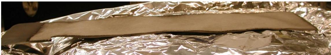
Fig. 4. FS1 U10Mo foil coated with Zr on both sides showing reduced curvature compared to the uncoated foil (Fig. 2).
