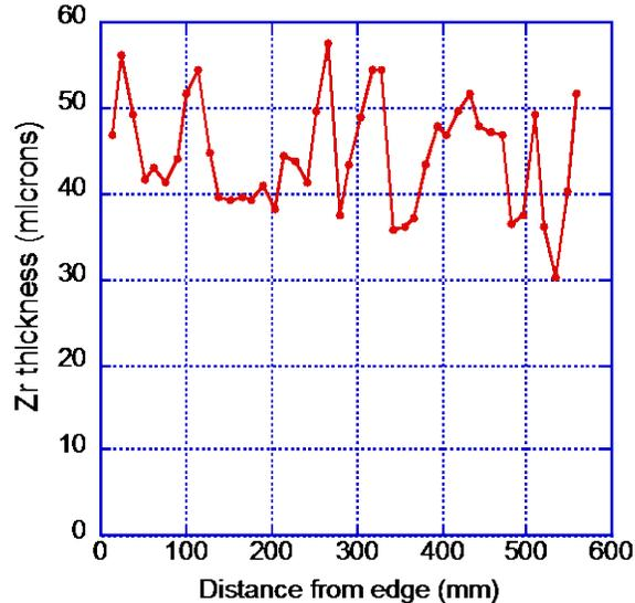
Fig. 14. XRF measurement of Zr coating thickness along the centerline of foil FS2.
