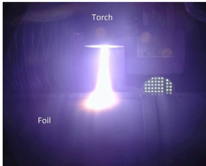
Fig. 6. Plasma torch spraying Zr powder onto the rotating fixture holding the FS2 U10Mo foil.
