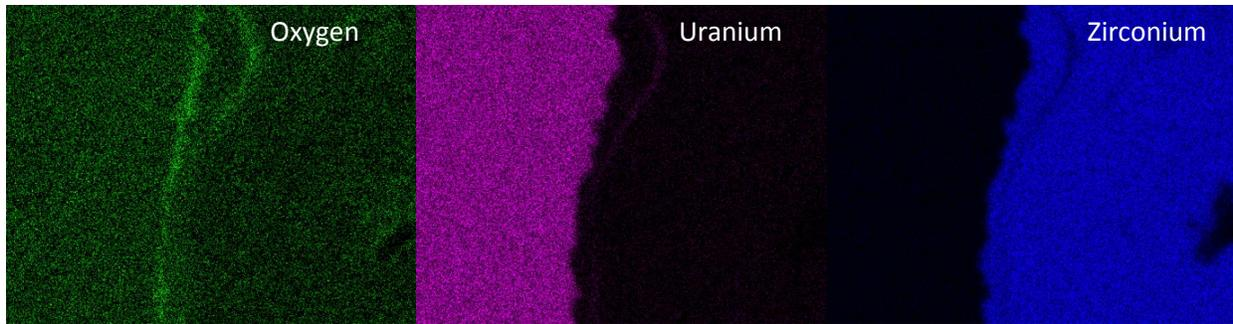
Fig. 10. Elemental maps of oxygen, uranium and zirconium for the area shown in Fig. 9.
