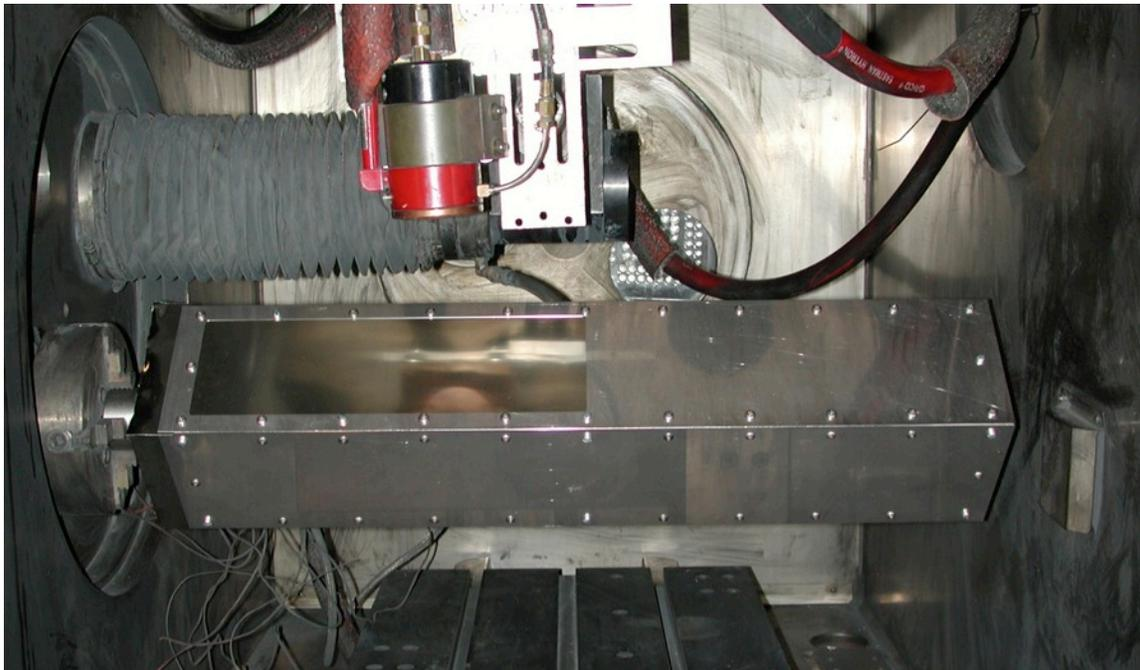
Fig. 1. Spinning foil holding fixture (lower center of image) mounted in the plasma spray chamber under the plasma torch (red on bottom and black on top).
