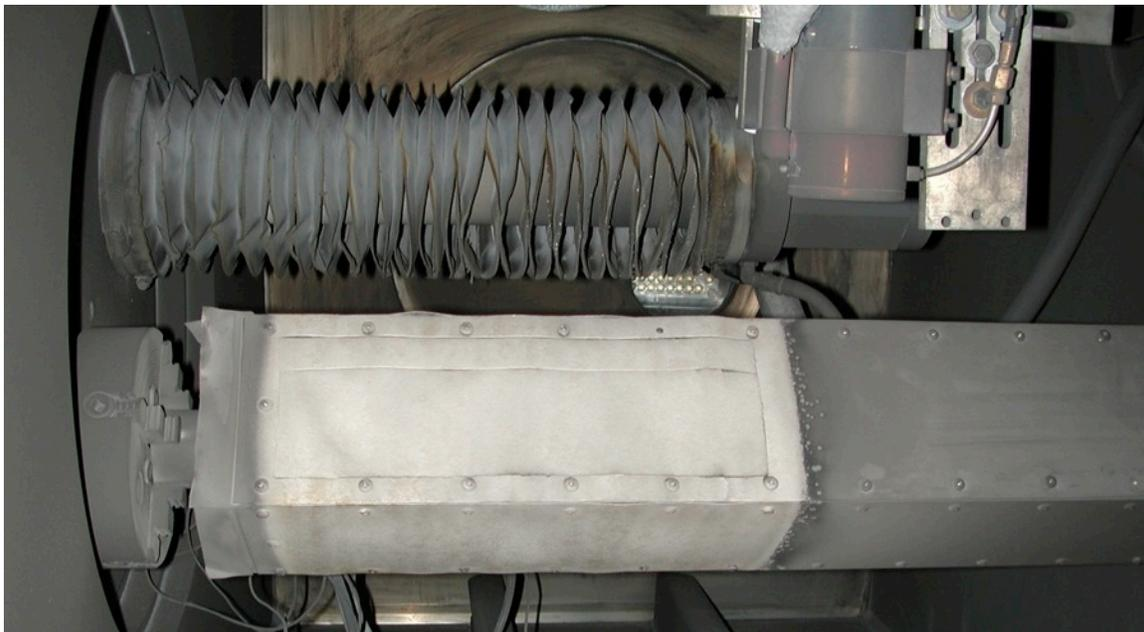
Fig. 3. FS1 U10Mo foil coated with Zr shown in the spray chamber attached to the rotating fixture.
