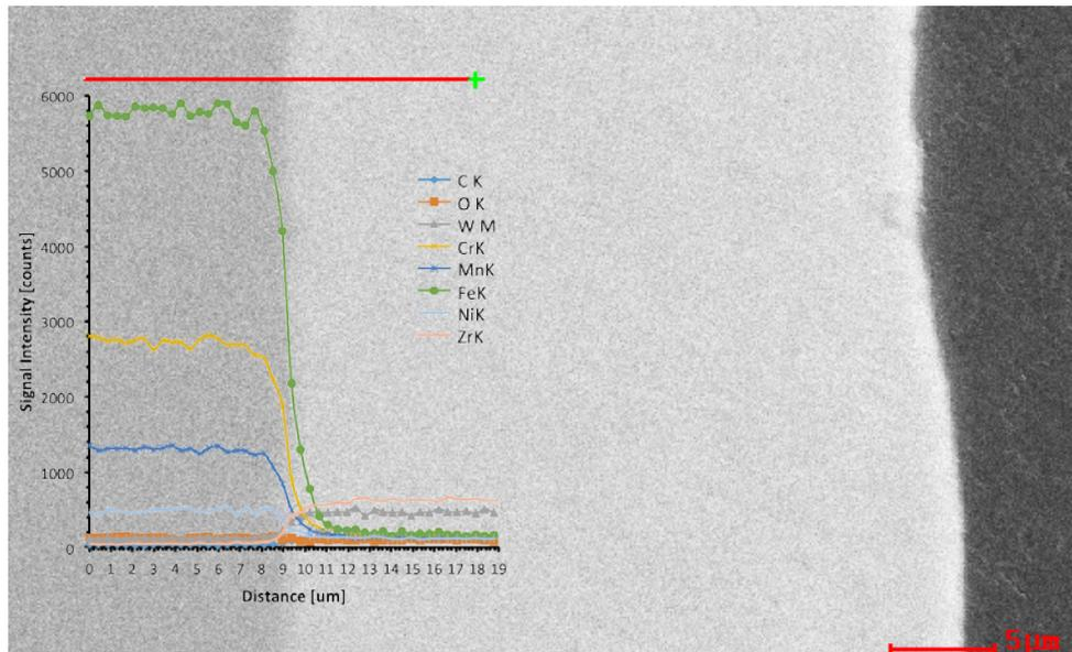
Fig. 13. SEM-BSE image and line scan (along the red line) elemental analysis of the cross section of a SS foil with a 30  $\mu\text{m}$  Zr foil resistance welded to the surface.
