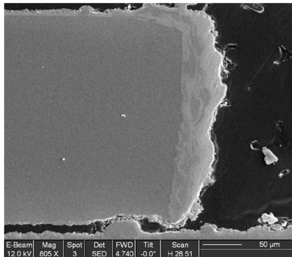
Fig. 11. Cross section of a stainless steel (left side) sample plasma sprayed on the edge with Zr (right side on edge of SS).
