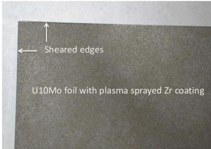
Fig. 8 Sheared edges of Zr plasma spray coated U10Mo FS1 foil.
