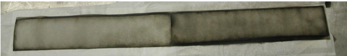
Fig. 7. FS2 U10Mo foil plasma spray coated with Zr. The dark line in the center of the sample shows the limits of the two separate spray runs needed to cover the entire top surface.
