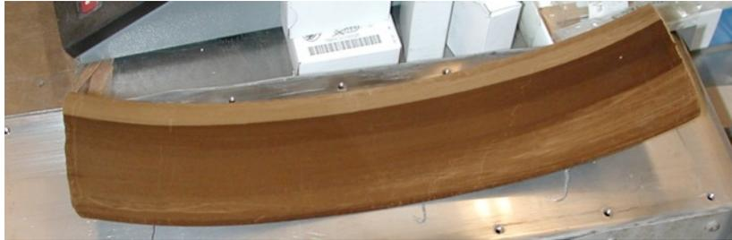
Fig. 2. FS1 U10Mo foil before coating showing significant curvature in the sample.
