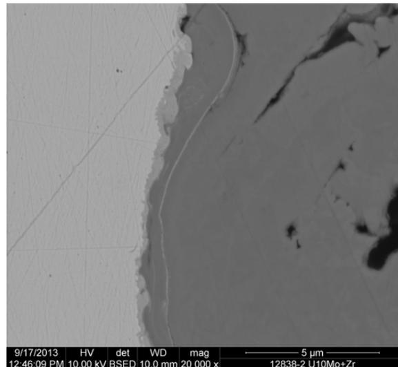
Fig. 9 SEM-BSE image of U10Mo (left side)/Zr (right side) interface in the FS1 foil.
