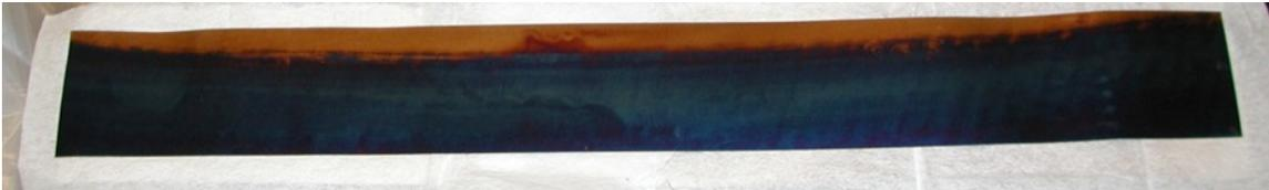
Fig. 5. FS2 U10Mo annealed foil prior to Zr coating.
