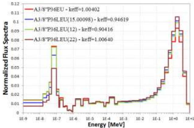
Figure 4. Central flux spectra in A3/8”P36EU and several A3/8”P36LEU
