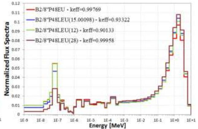
Figure 5. Central flux spectra in B2/8”P48EU and several B2/8”P48LEU
