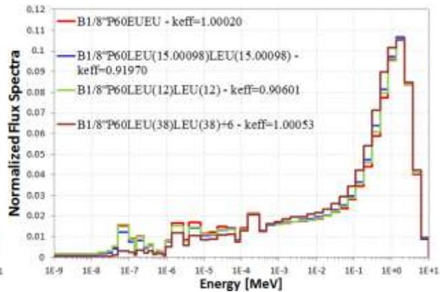
Figure 7. Central flux spectra in B1/8" P60EU-EU and several B1/8" P60LEU-LEU
