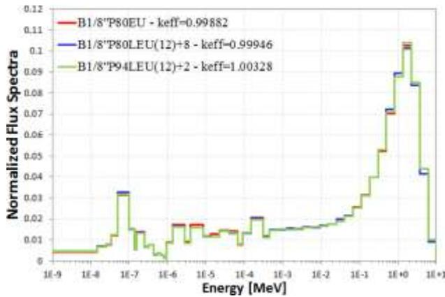
Figure 12. Central flux spectra in B1/8" P80EU, B1/8" P80LEU(12)+8 and B1/8" P94LEU(12)+2
