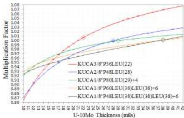
Figure 16. Sensitivity of KUCA LEU  $k_{eff}$  values to the tolerances of U-10Mo thickness
