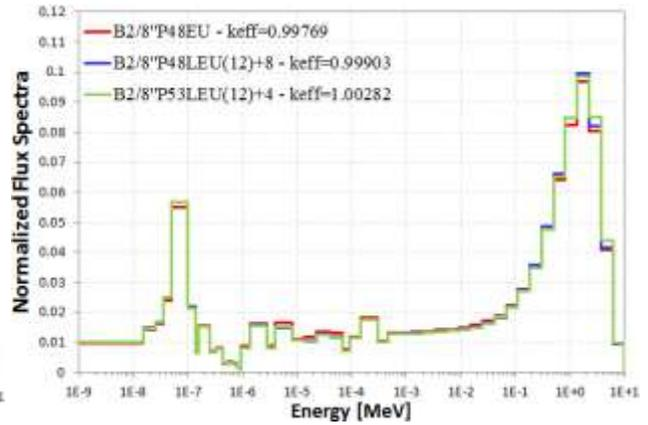
Figure 11. Central flux spectra in B2/8" P48EU, B2/8" P48LEU(12)+8 and B2/8" P53LEU(12)+4
