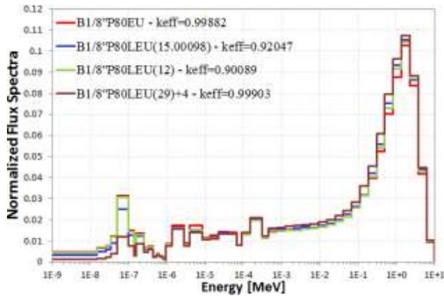
Figure 6. Central flux spectra in B1/8" P80EU and several B1/8" P80LEU
