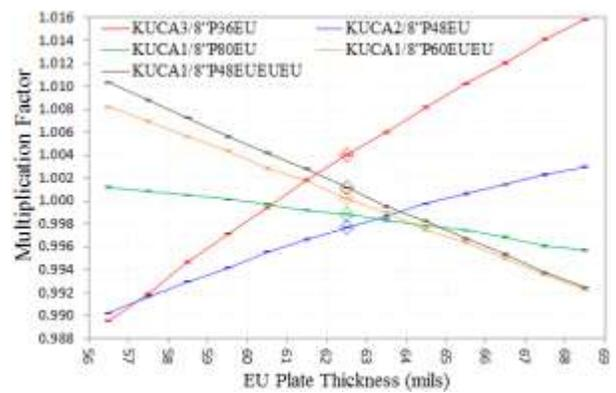
Figure 17. Sensitivity of KUCA HEU  $k_{eff}$  values to the tolerances of the fuel plate thickness
