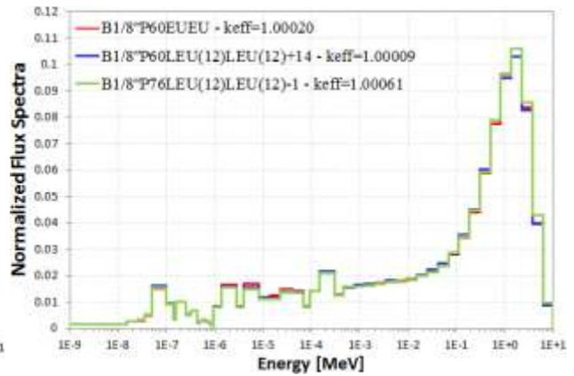
Figure 13. Central flux spectra in B1/8" P60EU-EU, B1/8" P60LEU(12)-LEU(12)+14 and B1/8" P76LEU(12)-LEU(12)-1
