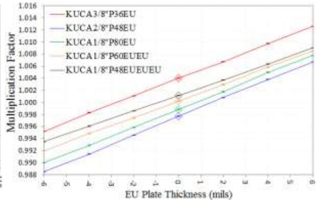
Figure 19. Sensitivity of KUCA HEU  $k_{eff}$  values to the tolerances of the fuel and polyethylene plate width
