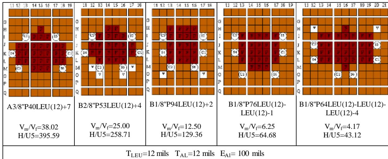
Figure 15. Layouts of the LEU KUCA cores using 12 mils thick U-10Mo foil and Al clad and reproducing about the same  $k_{eff}$  and central flux spectra of the corresponding HEU cores.
