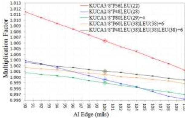
Figure 18. Sensitivity of KUCA LEU  $k_{eff}$  values to the tolerances of U-10Mo width
