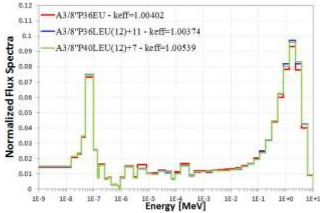
Figure 10. Central flux spectra in A3/8" P36EU, A3/8" P36LEU(12)+11 and A3/8" P40LEU(12)+7
