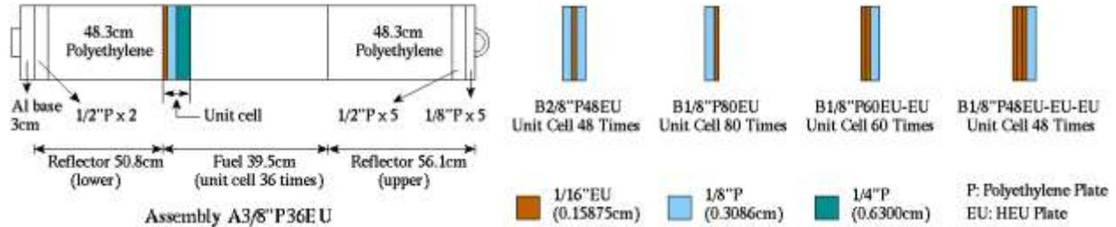
Figure 2. Cross sectional view of the KUCA fuel assemblies
