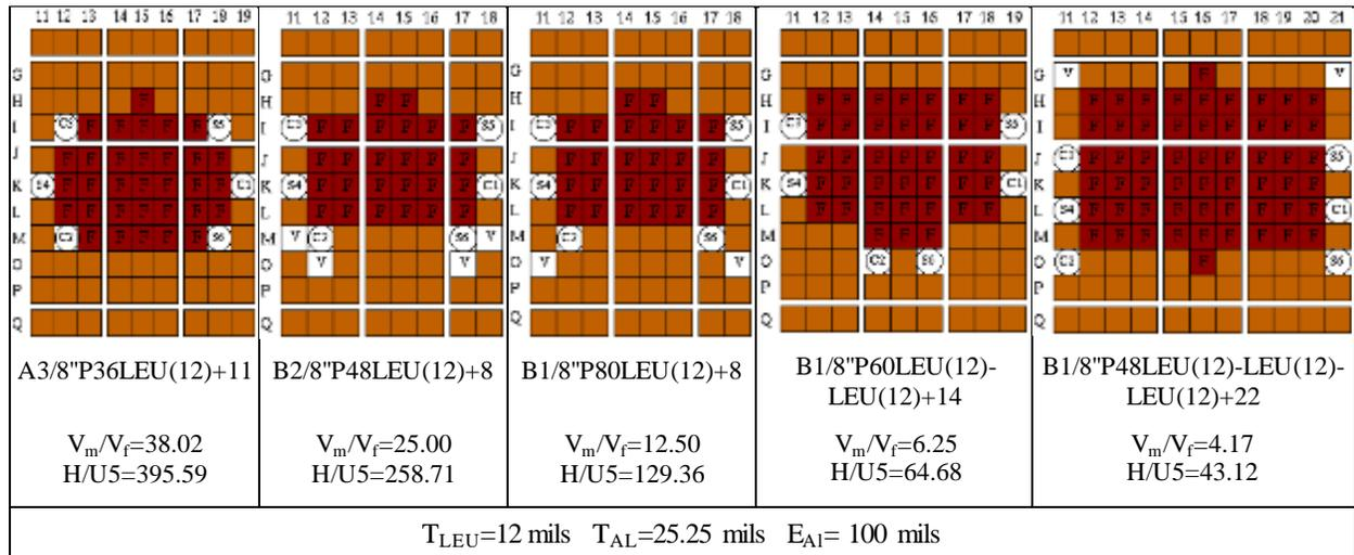
Figure 9. Layouts of the LEU KUCA cores reproducing about the same  $k_{eff}$  and central flux spectra of the corresponding HEU cores.
