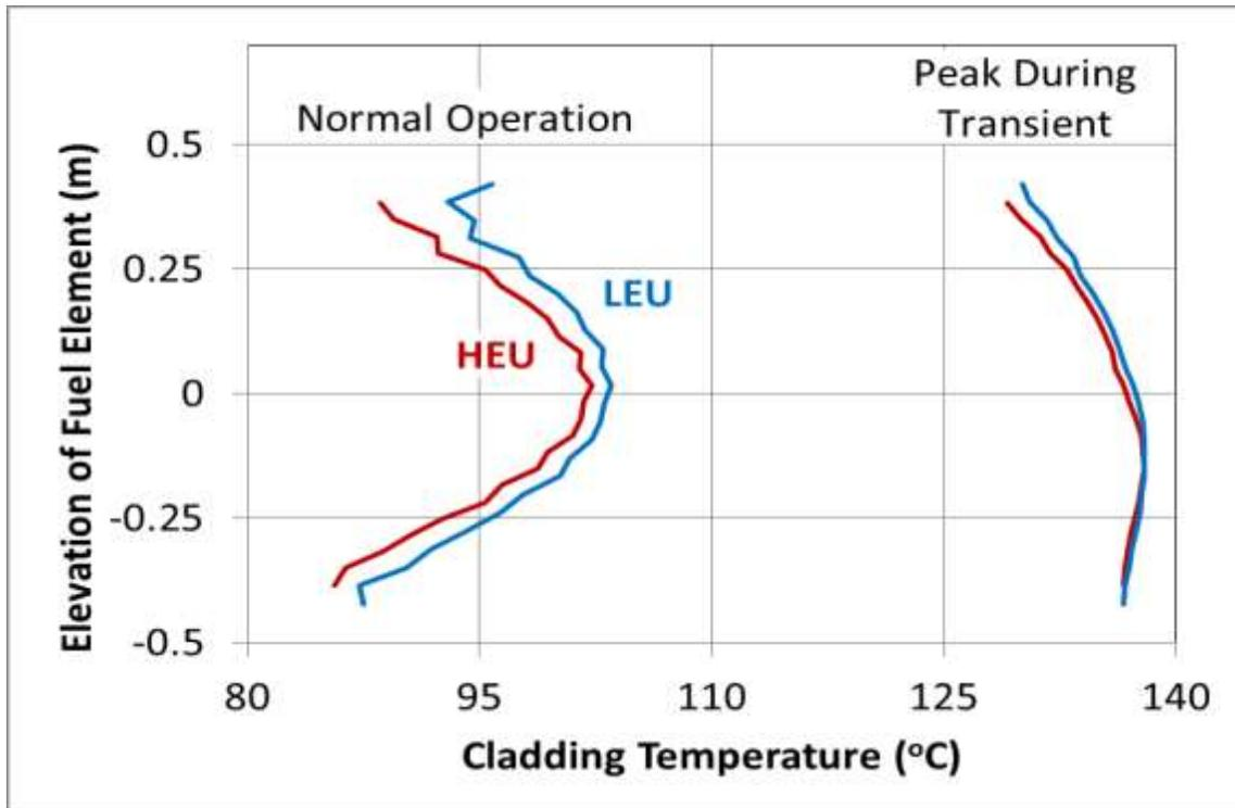
Figure 8. Cladding temperature comparisons for RELAP5 simulations with HEU and LEU fuel for the high heat flux heat structure (410).
