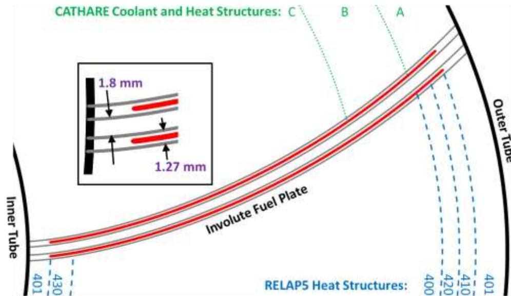
Figure 3. Conceptual drawing of the involute fuel plates (only 2 of 280 shown) and the CATHARE and RELAP5 discretization.
