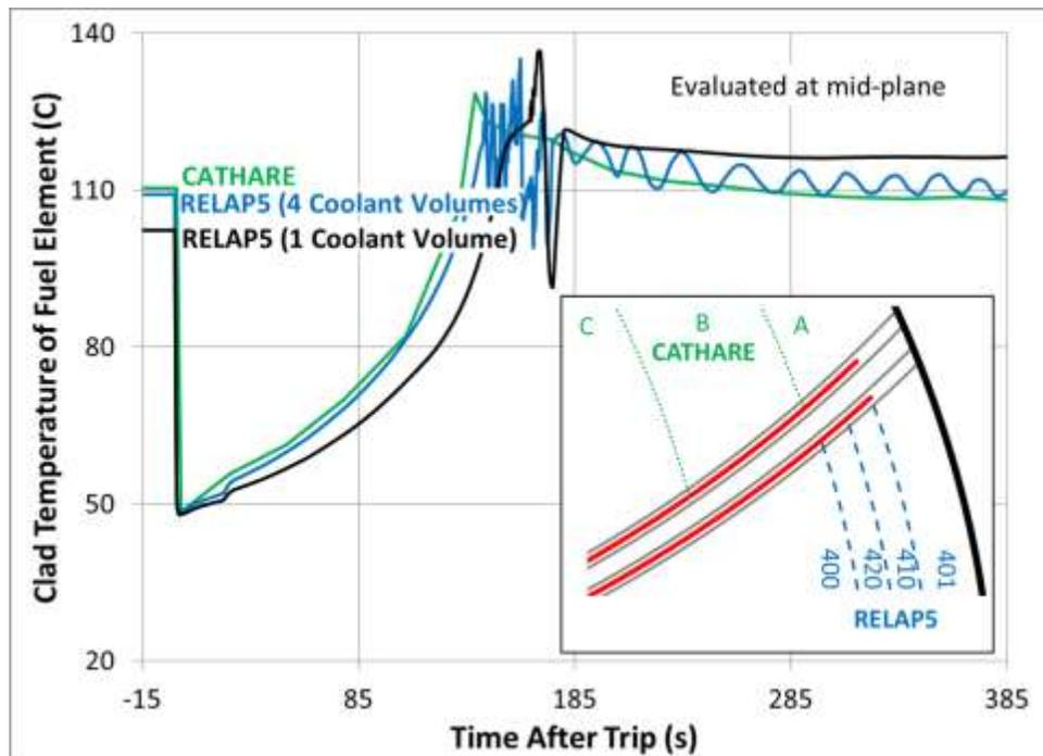
Figure 7. Mid-plane clad temperature at heat structures 410 (RELAP5) and A (CATHARE).
