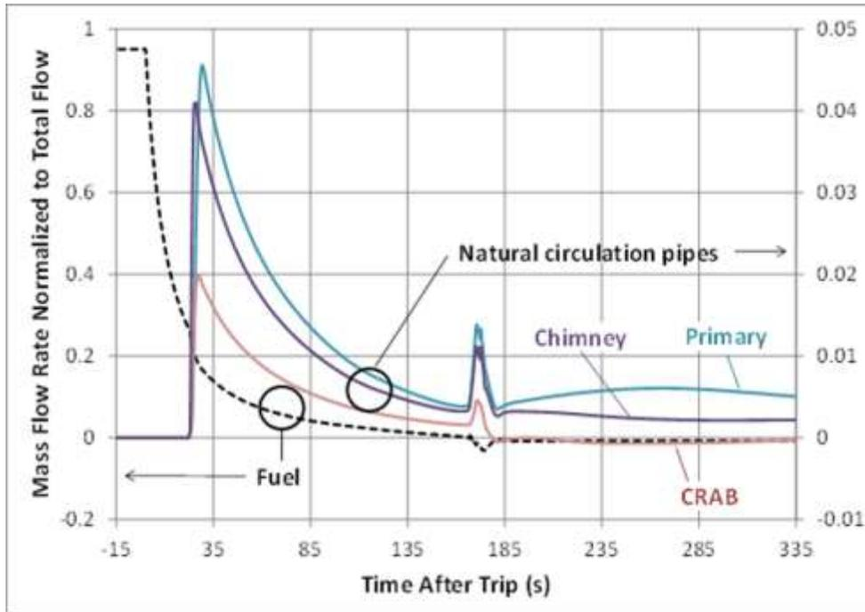
Figure 6. Mass flow rate through fuel and natural circulation pipes calculated by RELAP5 normalized to the total reactor flow rate.
