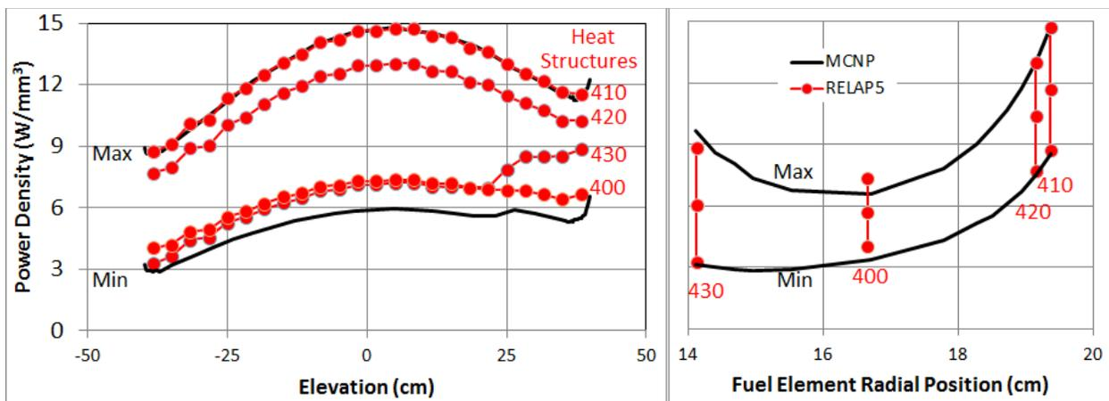
Figure 4. Axial and radial power density distribution at BOC (HEU fuel).
