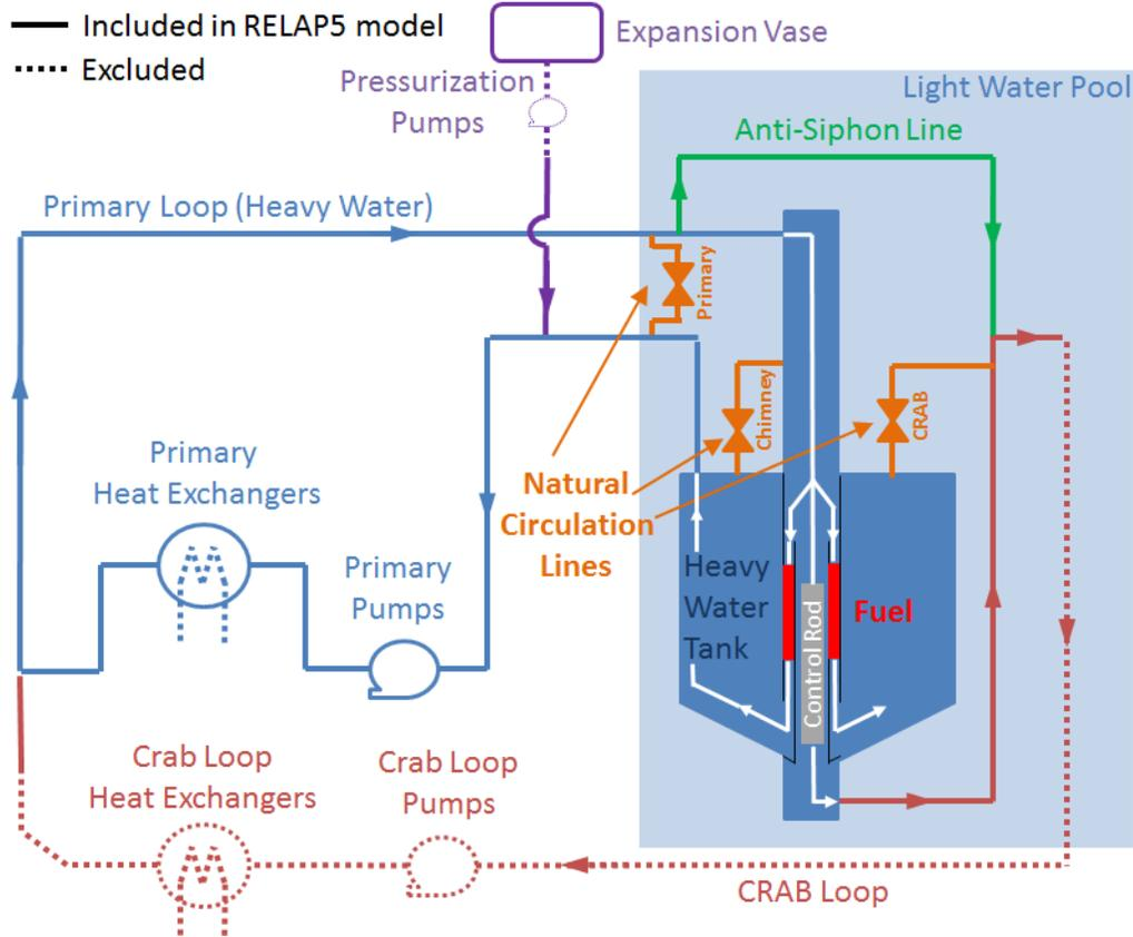
Figure 1. Conceptual drawing of RHF.
