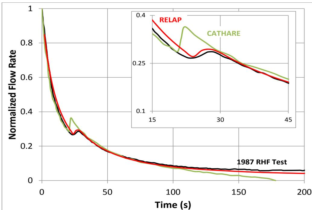
Figure 5. Comparison of the simulated and measured RHF pump coast down.
