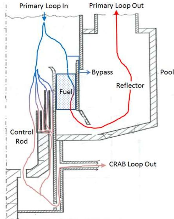
Figure 2. Axisymmetric drawing of the heavy water tank.
