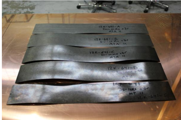
Figure 10 A series of cold rolled foils prepared for annealing at 650°C. have been placed on a Cu sheet. D. Alexander, K. Clarke
