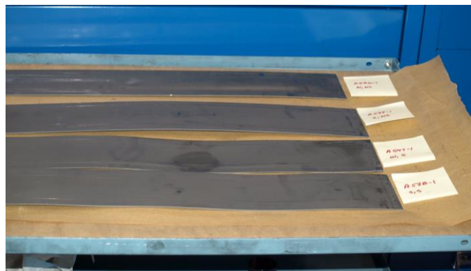
Figure 15 Photograph of plates after HIP. Plate 536-1 at the top has a bulge probably due to a leak in a weld during the HIP run. T. Lienert
