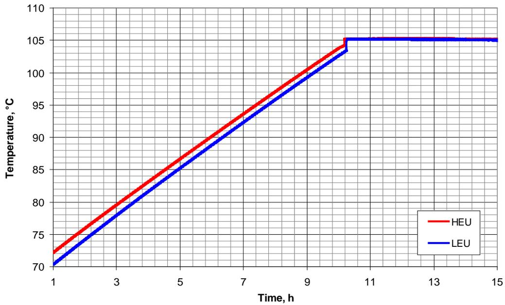
Fig. 10. Change in maximum coolant temperature in gap between the 1<sup>st</sup> and the 2<sup>nd</sup> fuel elements after pressure pipes rupture
