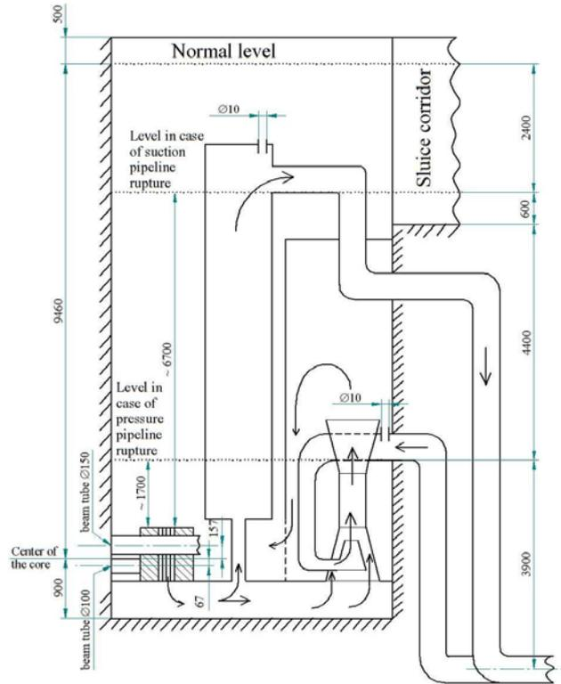
Fig. 2. Scheme of the reactor pool with pressure and suction pipes
