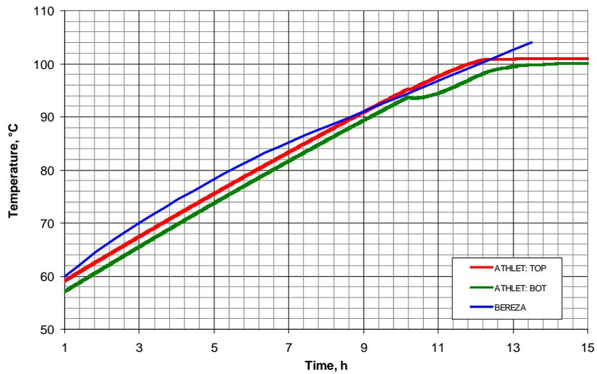
Fig. 11. Change in pool water temperature after pressure pipes rupture (HEU)
