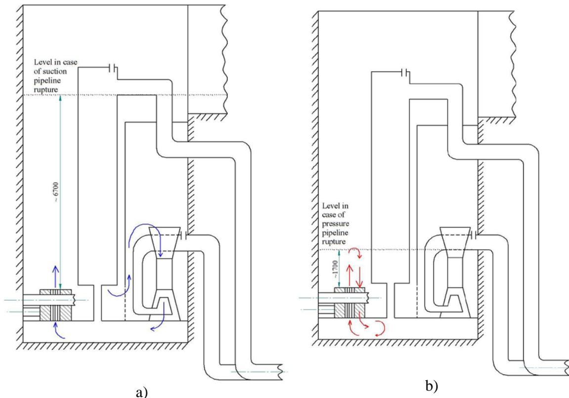
Fig. 5. Scheme of water movement at natural circulation:
