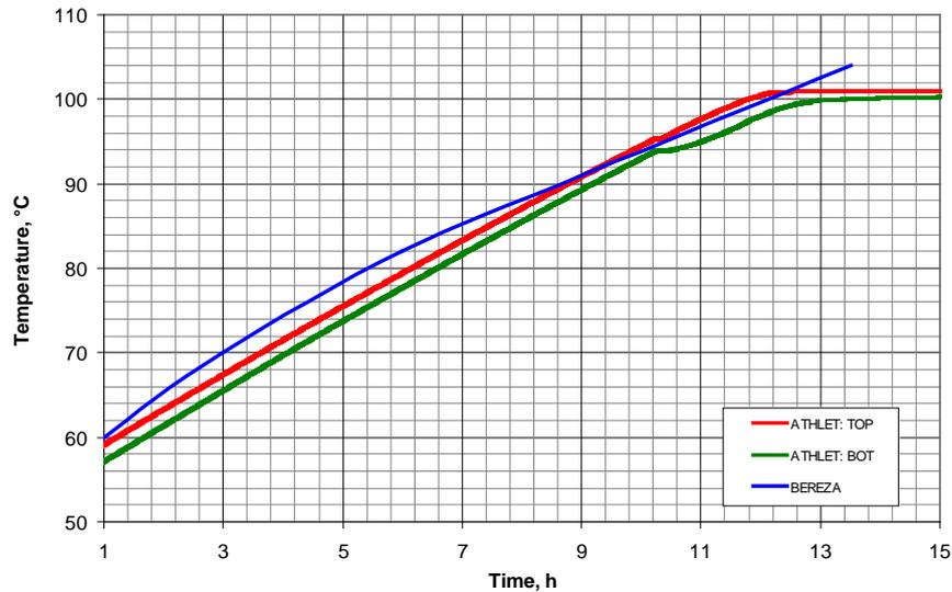
Fig. 12. Change in pool water temperature after pressure pipes rupture (LEU)
