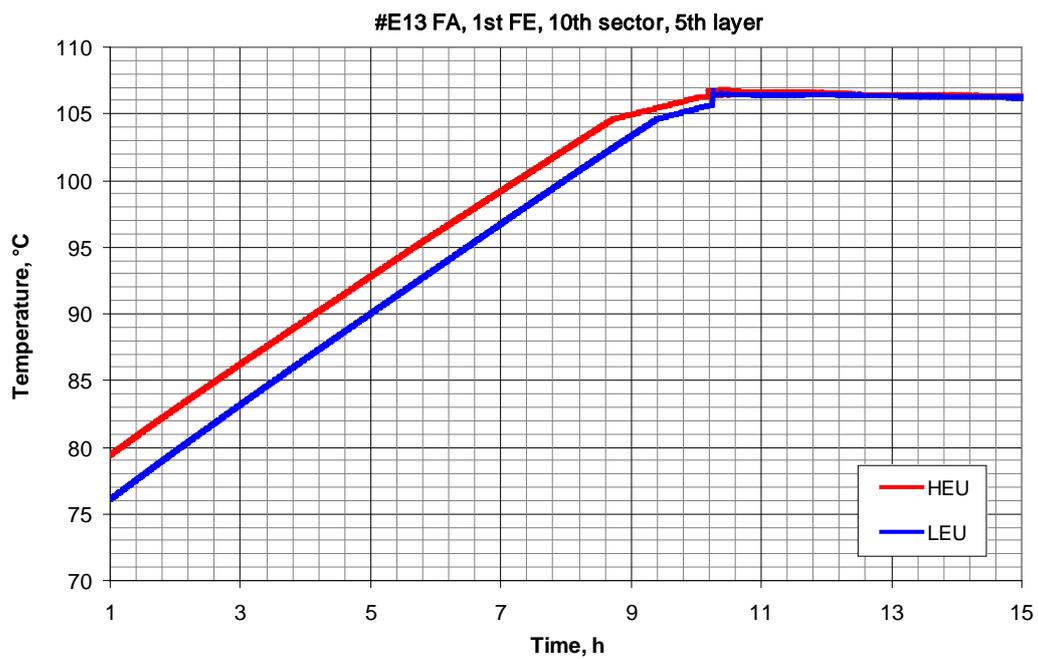
Fig. 9. Change in maximum fuel element inner surface temperature after pressure pipes rupture
