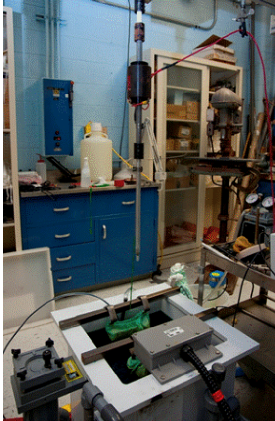
Fig. 5: Nickel electroplating bath for plating uranium metal foils
