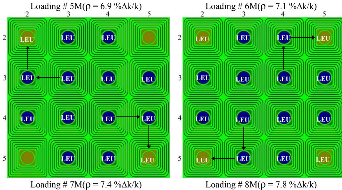
Figure 9. Principal scheme of the IR-8 reactor conversion to LEU fuel.
