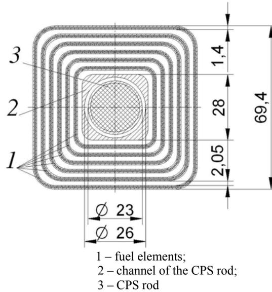
Figure 6. Cross section of IRT-3M FA with control rod
