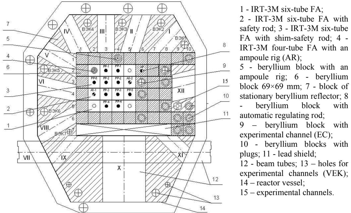
Fig 14. Cross section of the IR-8 core and of the reflector
