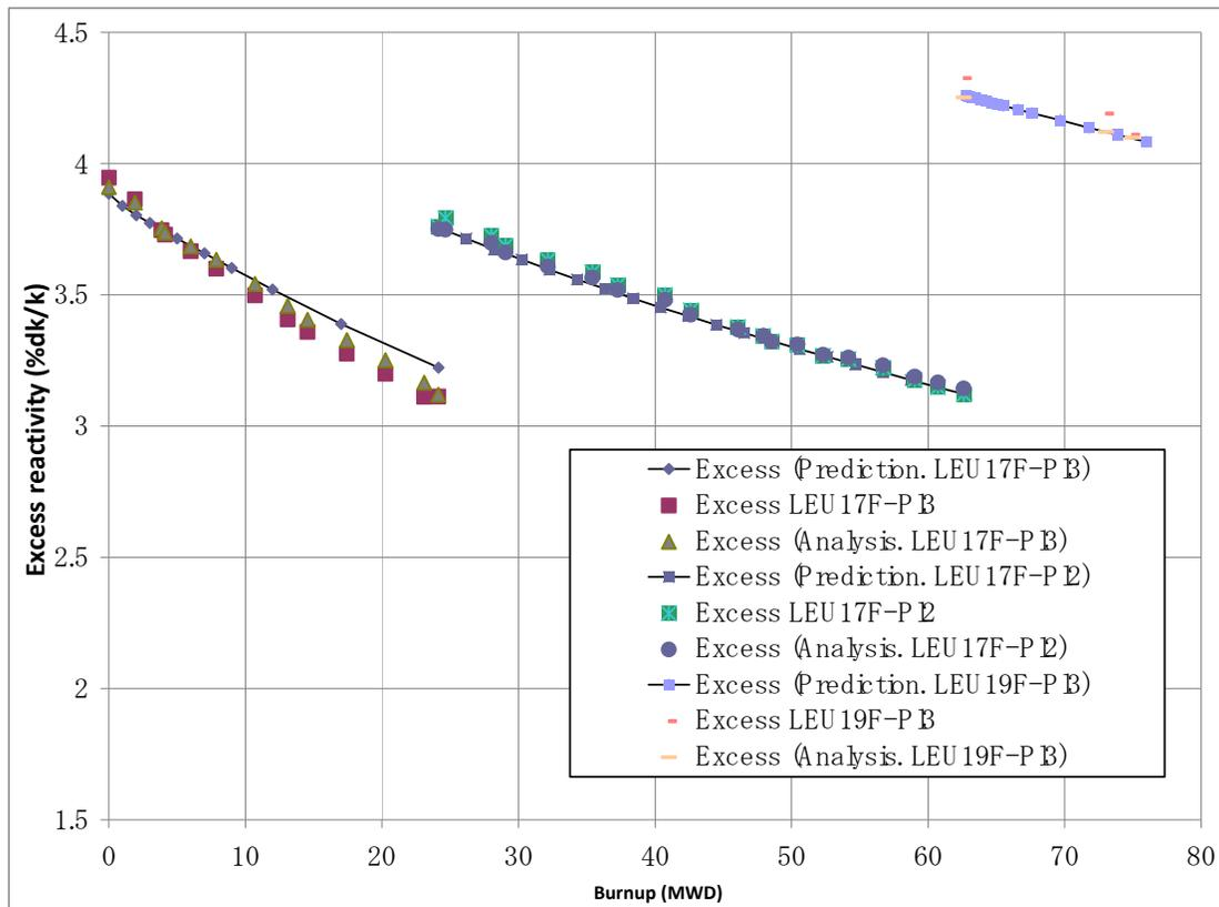
**Figure 14:** Burnup Dependence of Excess Reactivity
