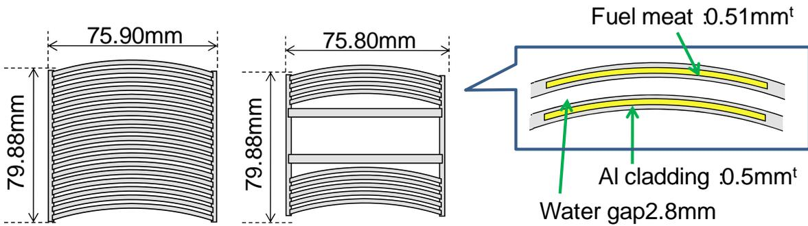
**Figure 4:** Cross section of fuel element and fuel plate
