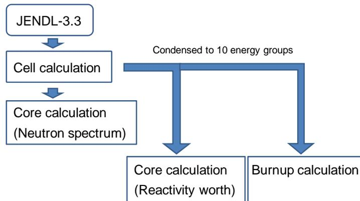
**Figure 9**: Calculation flow of KUR nuclear design
