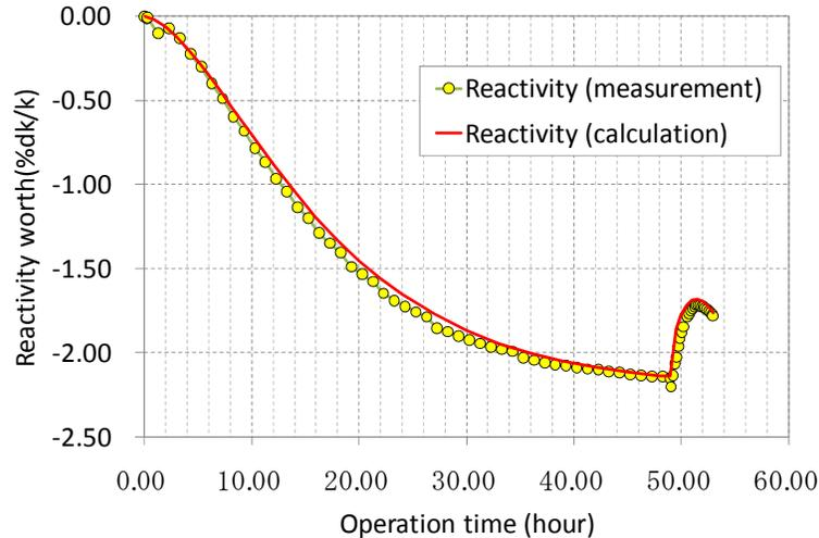
**Figure 11:** Burnup reactivity worth in 1 cycle operation
