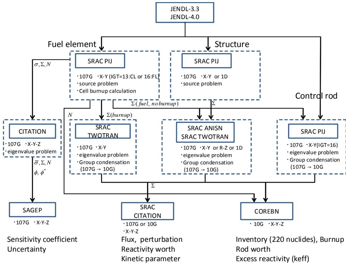
**Figure 12:** Detailed Calculation flow of KUR core management
