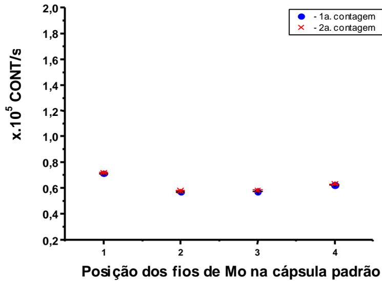
Figure 4. Reaction rates in the Mo wires inside the irradiation capsule filled with MoO<sub>3</sub> in the EIBe, channel A, and core position 65.
