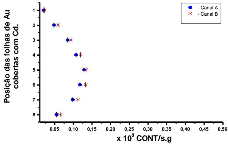
Figure 2. Reaction rates in the Au foils covered with Cd in the EIBe, channels A and B, and core position 65.
