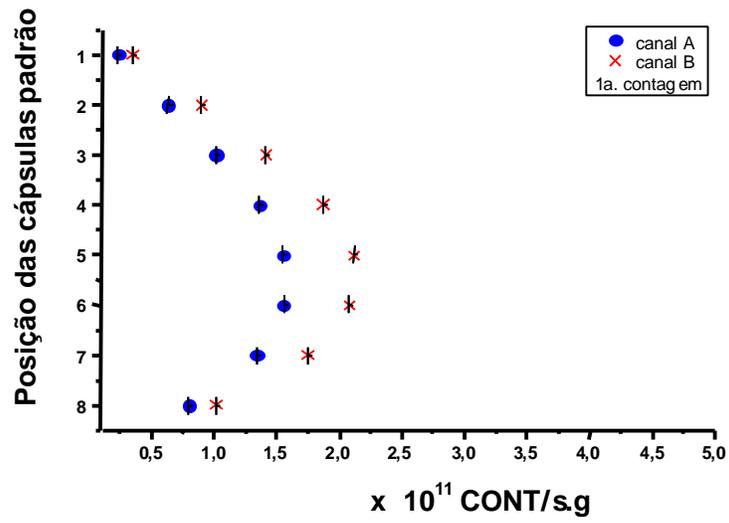
Figure 1. Reaction rates in the In foils covered with Cd in the EIBe, channels A and B, and core position 45.
