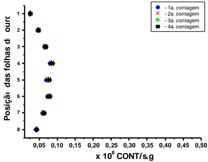
Figure 3. Reaction rates in the Au foils covered with Cd in the EIGRA, channels A and B, and core position 65.
