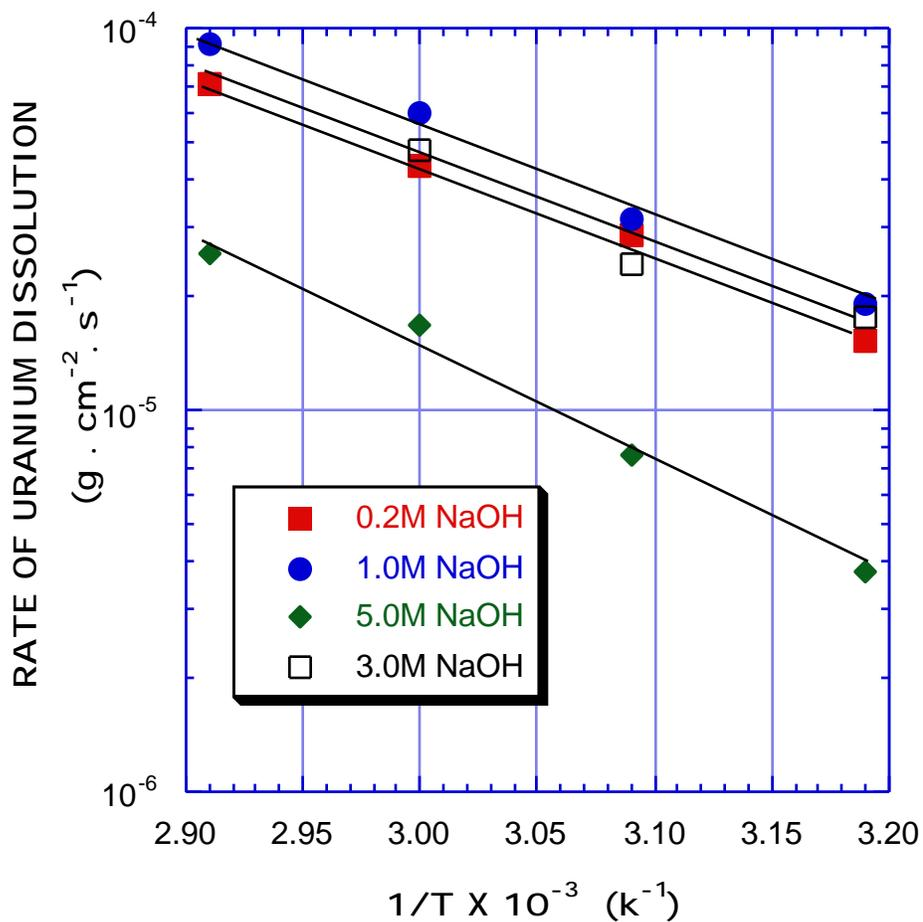
Figure 5. Effect of Temperature on Rate of Uranium Dissolution (U Surface 2.0 cm<sup>2</sup>, Initial [H<sub>2</sub>O<sub>2</sub>] 4.0M)
