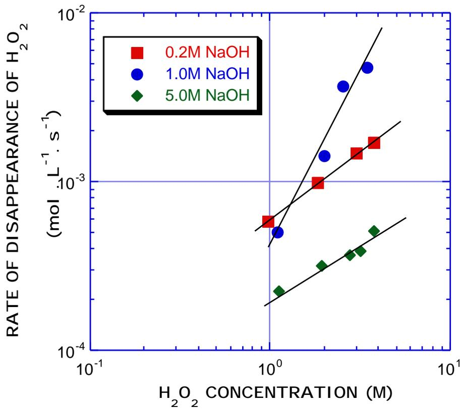
Figure 4. Effect of Hydrogen Peroxide on Rate of Its Depletion (U Surface 2.0 cm<sup>2</sup>, Temp.=60°C)
