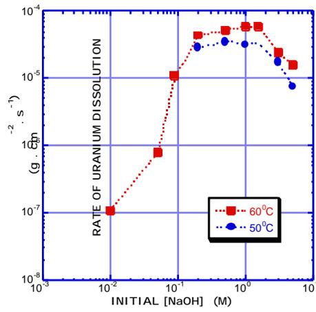
Figure 1. Effect of Initial Alkaline Concentration on Rate of Uranium Dissolution (U Surface 2.0 cm<sup>2</sup>, Initial [H<sub>2</sub>O<sub>2</sub>] 3.5M)
