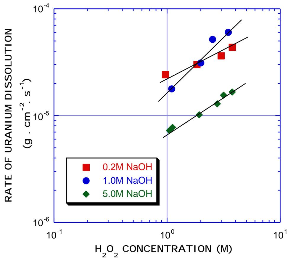
Figure 3. Effect of Hydrogen Peroxide on Rate of Uranium Dissolution (U Surface  $2 \text{ cm}^2$ , Temp. $=60^\circ C$ )
