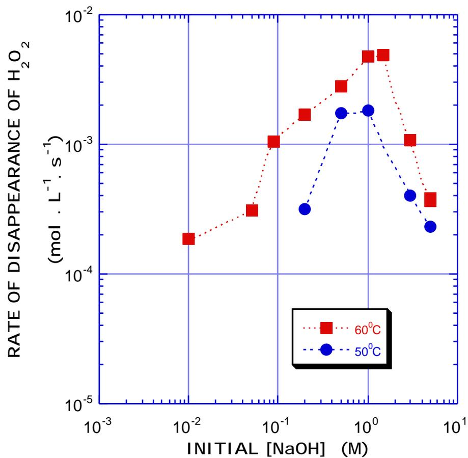
Figure 2. Effect of Alkaline Concentration on Rate of Depletion of H<sub>2</sub>O<sub>2</sub> (U Surface 2.0 cm<sup>2</sup>, Initial[H<sub>2</sub>O<sub>2</sub>] 3.5M)
