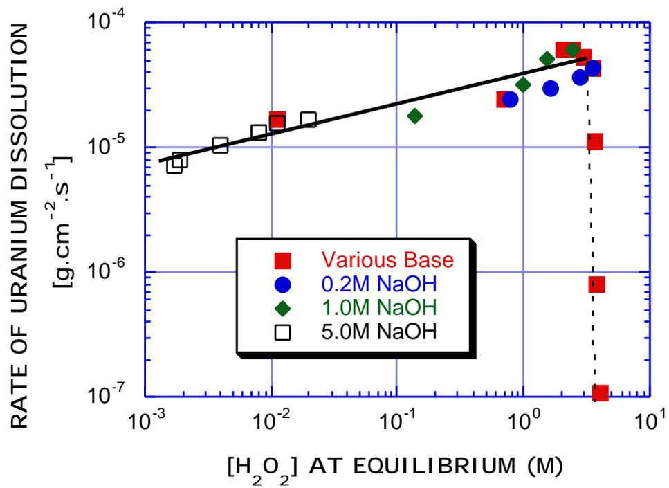
Figure 7. Effect of Equilibrium Hydrogen Peroxide Concentration on Rate of Uranium Dissolution (U Surface = 2 cm<sup>2</sup>, Temp. = 60°C)
