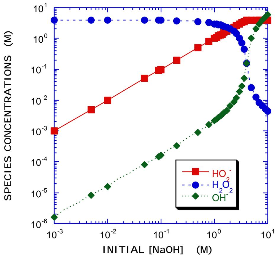
Figure 6. Effect of Hydroxide Concentration on  $\text{H}_2\text{O}_2$  Equilibrium (Initial  $[\text{H}_2\text{O}_2] = 4.0\text{M}$ )
