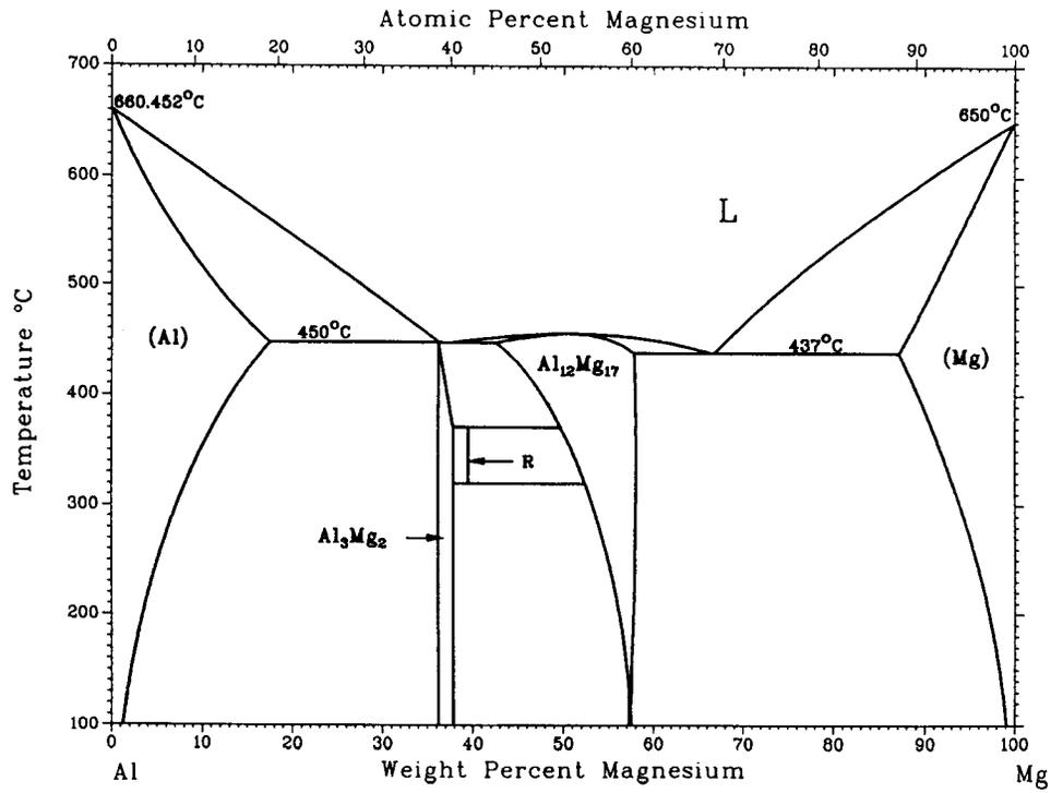
Fig. 3. Al-Mg phase diagram.
