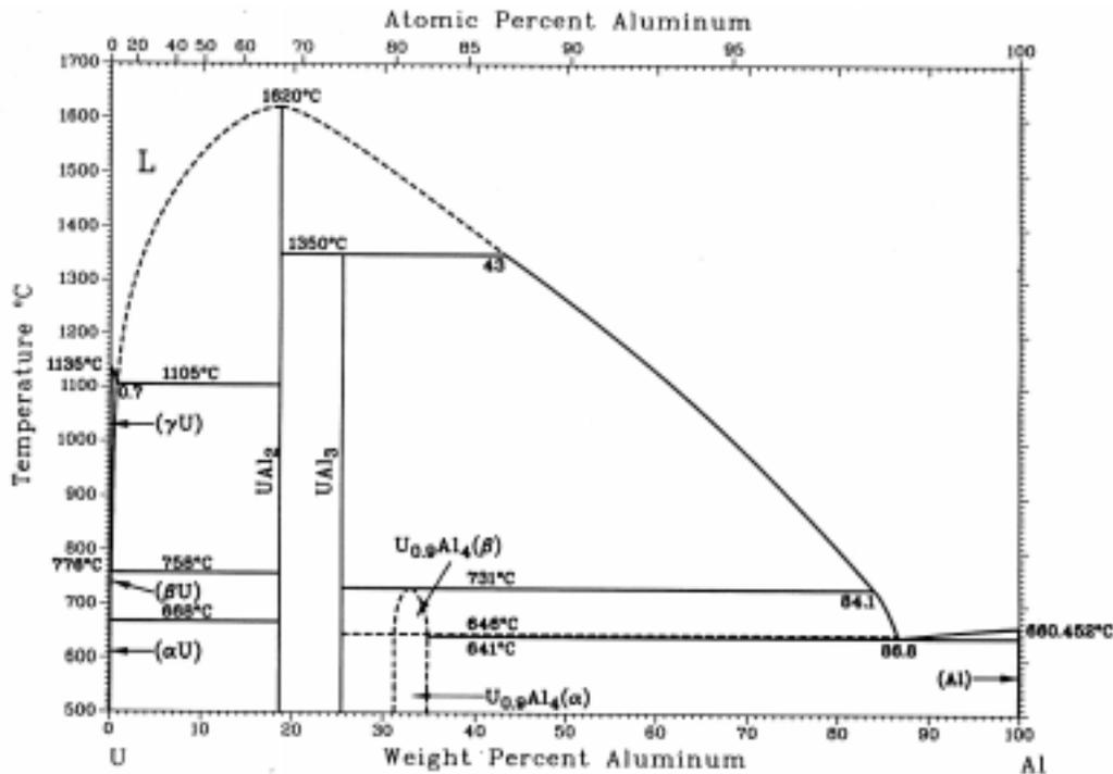
Fig. 1. U-Al phase diagram.
