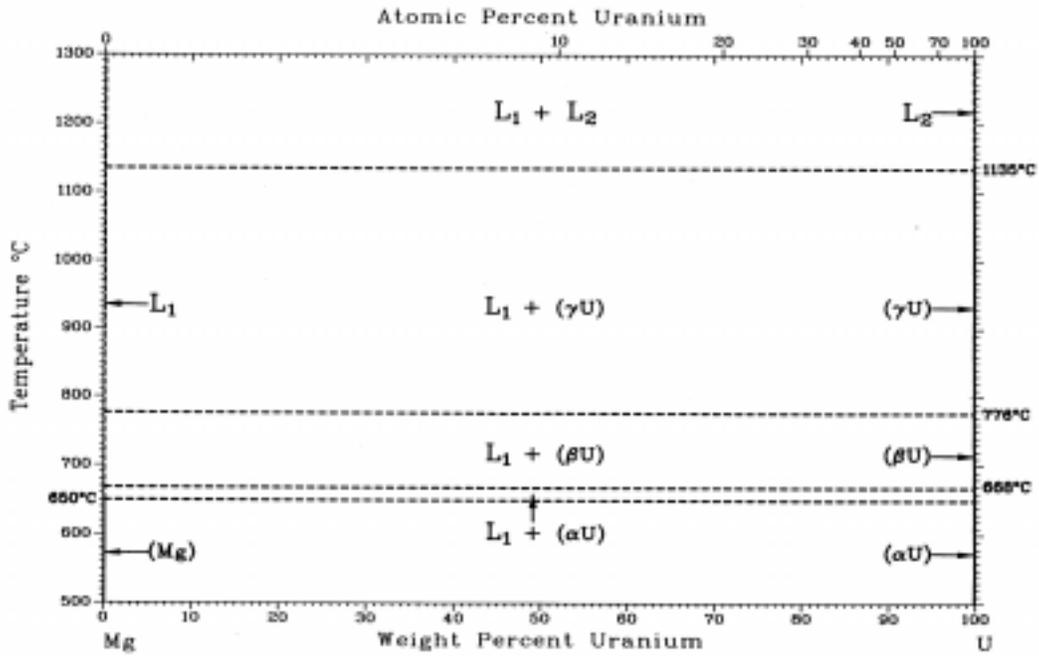
Fig. 2. U-Mg phase diagram.
