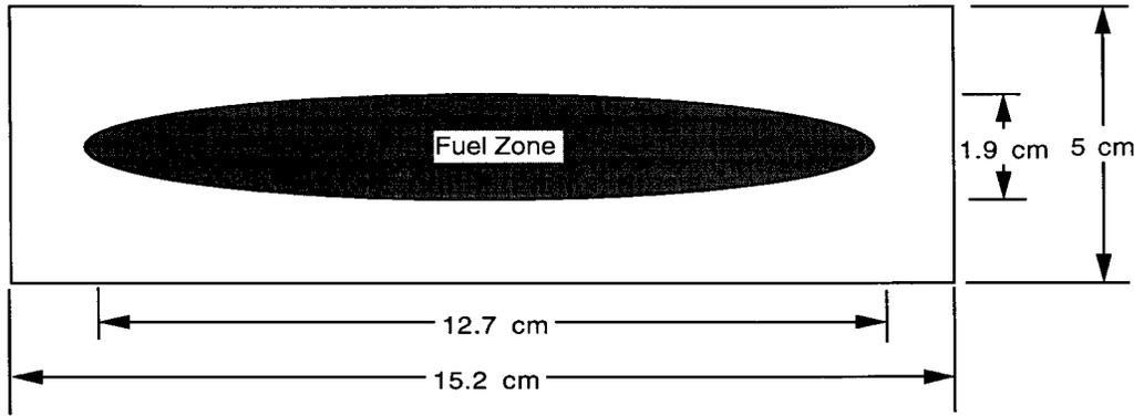
Fig. 4. Design of fuel plate for bonding and compatibility study experiments.
