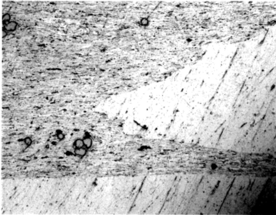
Fig. 7. Interface between 6061-Al-clad Mg-matrix processed at 275°C;  $\approx 200 \times$ .
