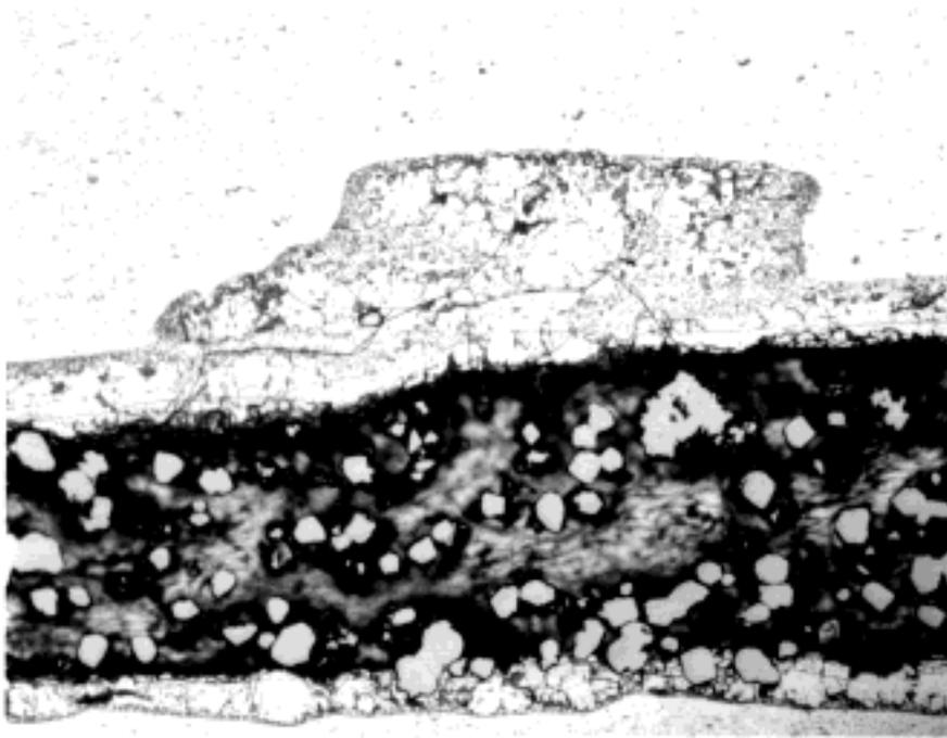
Fig. 6. Diffusion zones for 6061-Al-Mg-matrix processed at 415°C;
