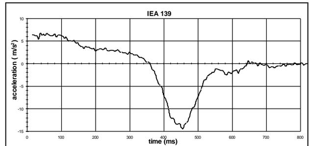
Figure 8 - Control Rod Drop Acceleration
