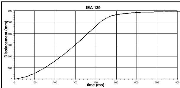
Figure 6 – Control Rod Drop Displacement
