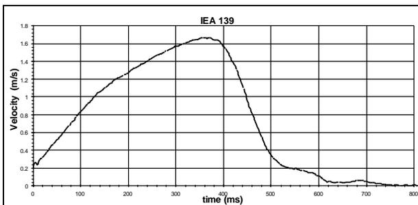
Figure 7 - Control Rod Drop Velocity
