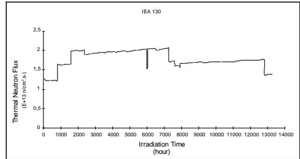
Figure 1. Average Thermal Flux for IEA-130.
