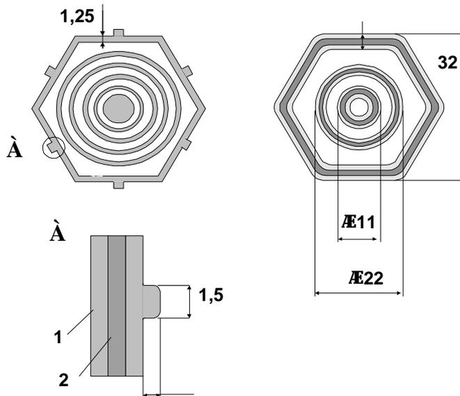
Figure 4. Cross-Sections of Fuel Assemblies of the WWR-M2 type (right) and WWR-M5 type (left). 1 – plating. 2 - nuclear fuel layer
