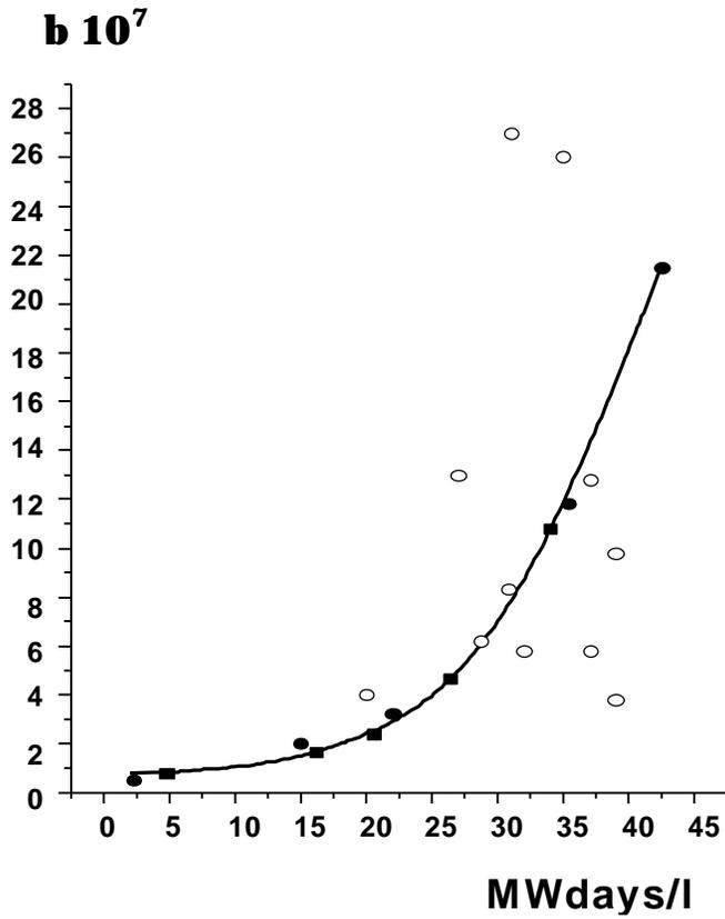
Figure 3. Relation of mean non-integrity  $\beta$  to specific energy release for two types of fuel elements: ■ -WWR-M2 and ● -WWR-M5 and ○ -  $\beta$  values for individual fuel elements.
