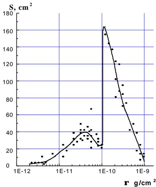
Figure 2. Uranium 235 Density Distribution Across Fuel Element Surface
